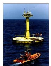
Figure 4: 10-Meter Discus-Shaped Hull Buoy Source: NDBC (2012)
