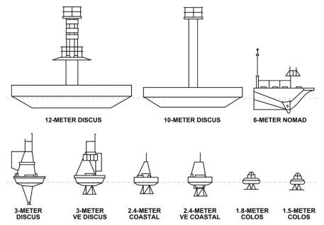
Figure 3: Buoy Schematic Source: NDBC (2008)
