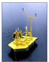
Figure 5: 6-Meter Boat-Shaped Hull Buoy Source: NDBC (2012)
