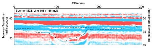
Boomer data is typically not useful in mapping reflectors less than 5 meters below the seafloor due to limited vertical resolution.
