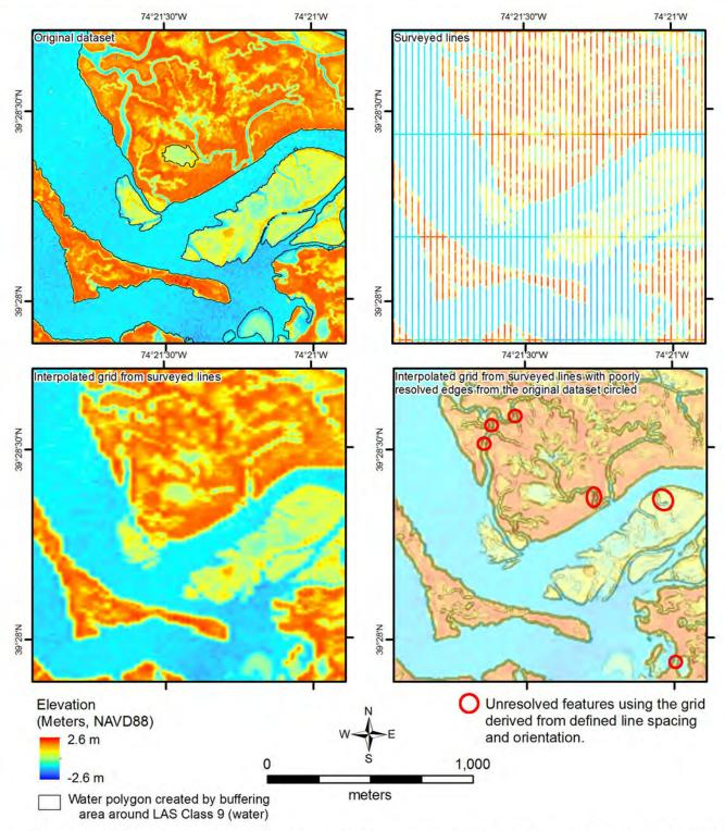
Note: The elevation data used for the 30 by 500 meter line spacing analysis came from a LiDAR DEM (RAMPP, 2011). LiDAR acquisition and processing to bare-earth was conducted by Fugro EarthData, Inc. The cell size of the above gridded DEM is approximately 6 by 6 meters. The tighter cell size allows smaller features to be resolved which is necessary for analyzing the 30 meter line spacing, although the areas at or below water level are not accurate topographic elevations.
