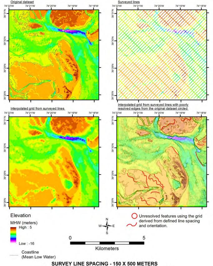
SURVEY LINE SPACING - 150 X 500 METERS NORTHEAST-SOUTHWEST PRIMARY LINE ORIENTATION
