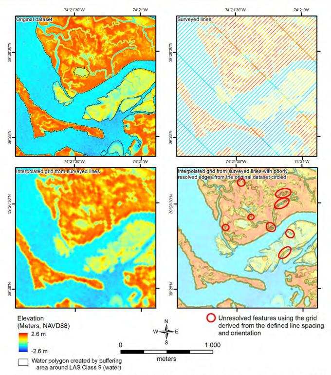
Note: The elevation data used for the 30 by 500 meter line spacing analysis came from a LiDAR DEM (RAMPP, 2011). LiDAR acquisition and processing to bare-earth was conducted by Fugro EarthData, Inc. The cell size of the above gridded DEM is approximately 6 by 6 meters. The tighter cell size allows smaller features to be resolved which is necessary for analyzing the 30 meter line spacing, although the areas at or below water level are not accurate topographic elevations.
