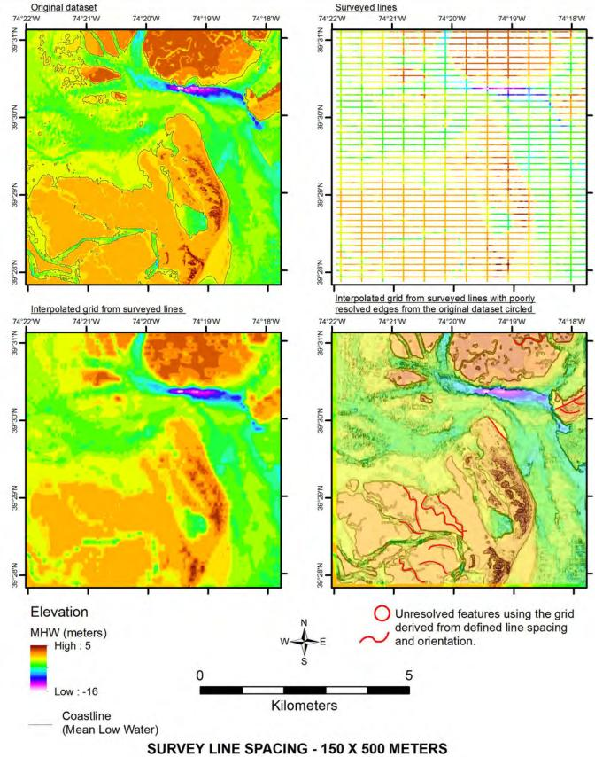
SURVEY LINE SPACING - 150 X 500 METERS EAST-WEST PRIMARY LINE ORIENTATION
