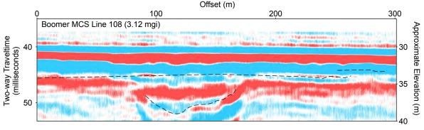
The two uppermost reflectors from the Chirp data are not as well-defined in the 3.12-mgi data. The shape of the deeper channel's thalweg is not as well-delineated using the 3.12-mgi data. Compared to the 1.56-mgi data, the channel's margins are not as well-defined and the erosional base cannot be mapped across the profile.
