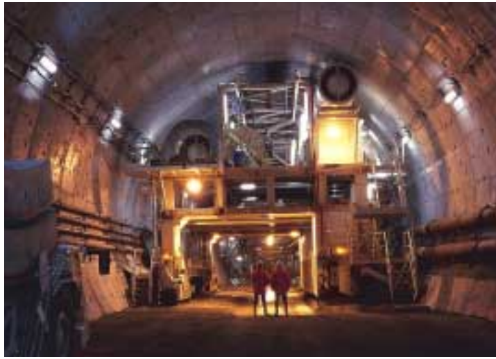
The Groene Hart (Netherlands) tunnel boring machine is the largest in the world: 14.85 metres in diameter.
