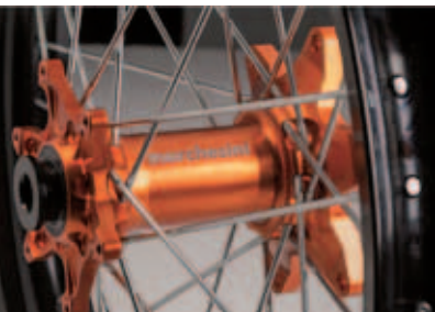
Marchesini motorbike wheels. Detail of the Rock spoked wheel for cross-country motorbikes.
