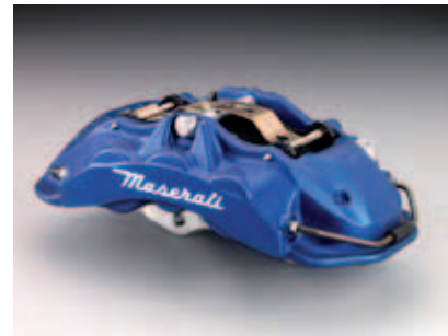
Cars. Front brake caliper on the Maserati GranTurismo Sport.
