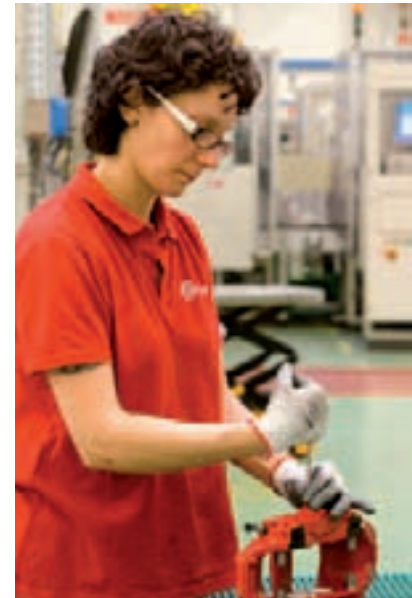
Curno car plant (Italy). Assembly of a caliper.
