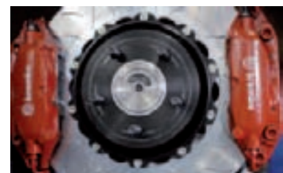
Disc with 4-piston high-performance double caliper fitted on the 1969 Dodge Charger Daytona, star of the film Fast & Furious 6.
