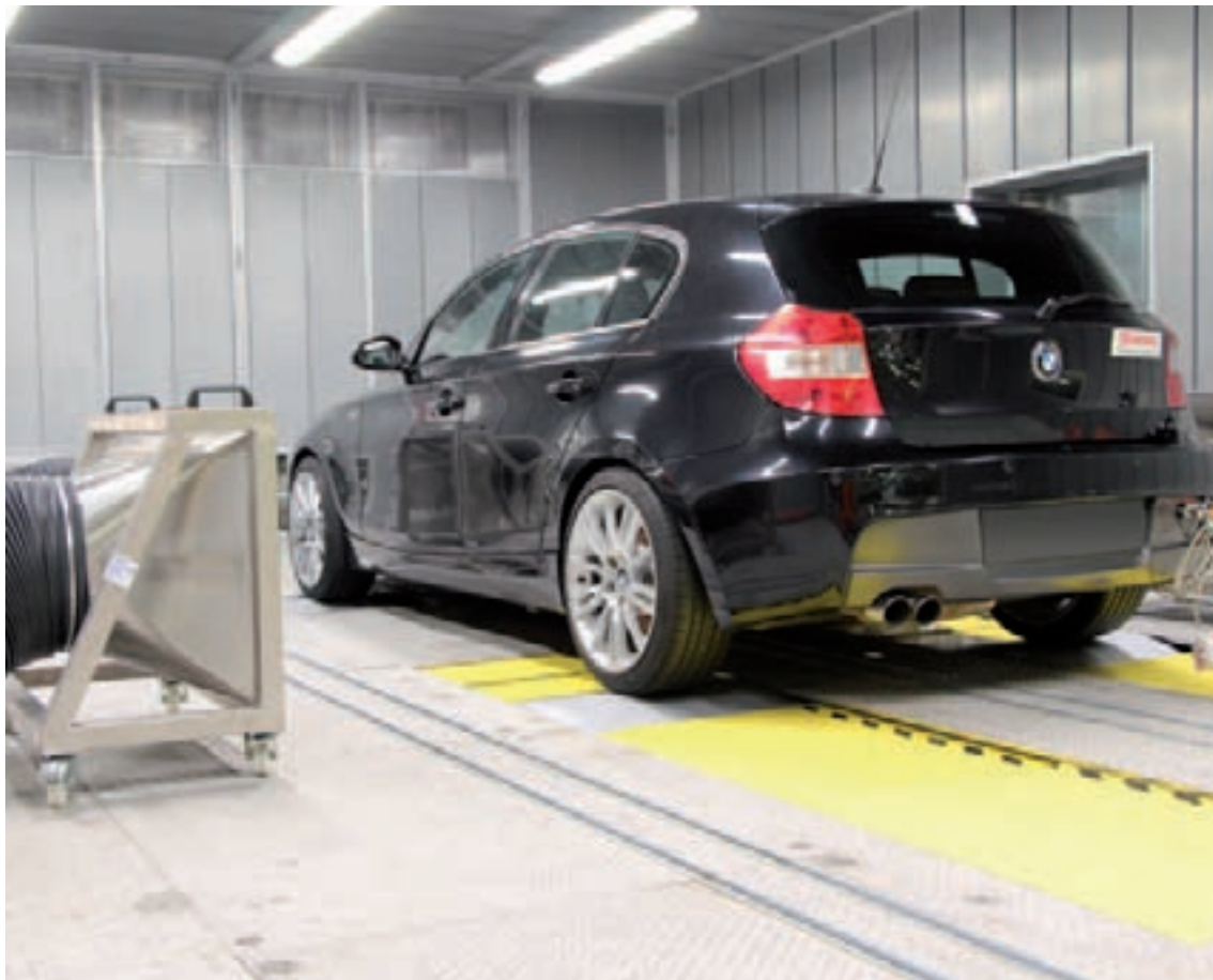
Testing Department in Stezzano (Italy). New dynamic roller test bed.
