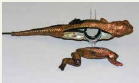
Photo showing steps in the construction of an anatomically accurate Te thermometer with an internal temperature logger. from Bakken and Angilletta's Perspective article
