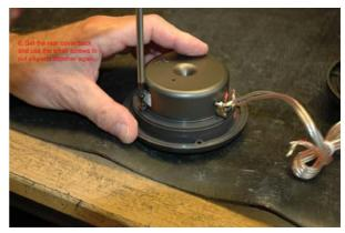
6. Reinstall the rear chamber and use the screws to put all parts together again.
