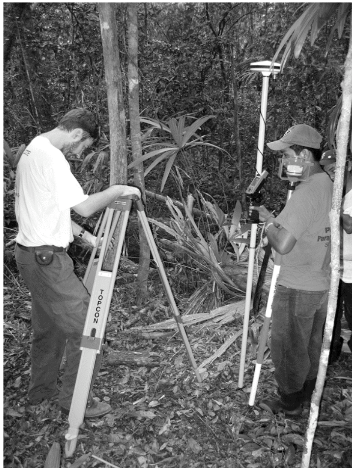
Figure 3.20. Transferring the GPS from the Rover Rod to the tripod (photo by Trevor Emond).
