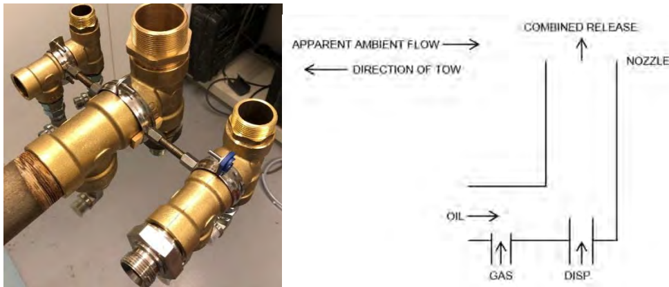
Figure 4. Photograph of the three-nozzle system and schematic of the release arrangement for each nozzle.
