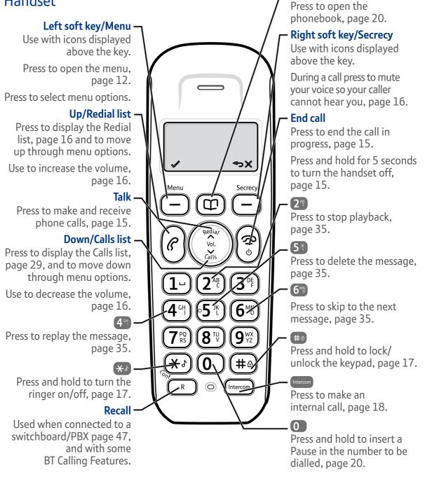
The answer machine handset controls on buttons 2<sup>4</sup> 4<sup>4</sup> 5<sup>4</sup> and 6<sup>4</sup> will only work when a message is being played on the handset, page 35.
