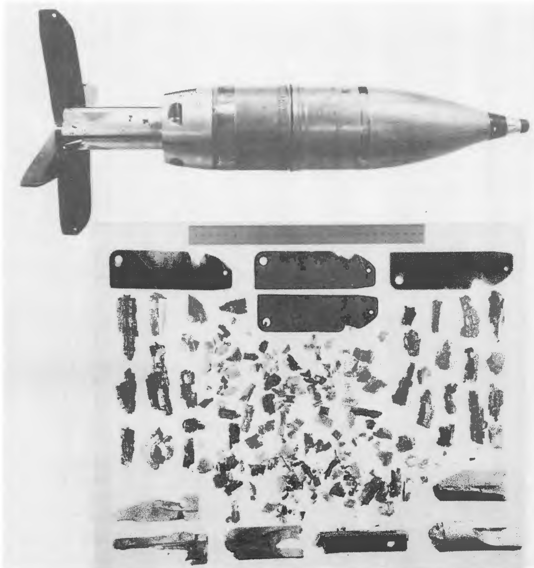
Figure 1-4. Russian 115-mm Fragments From Model OF-18 Frag-HE Projectile
