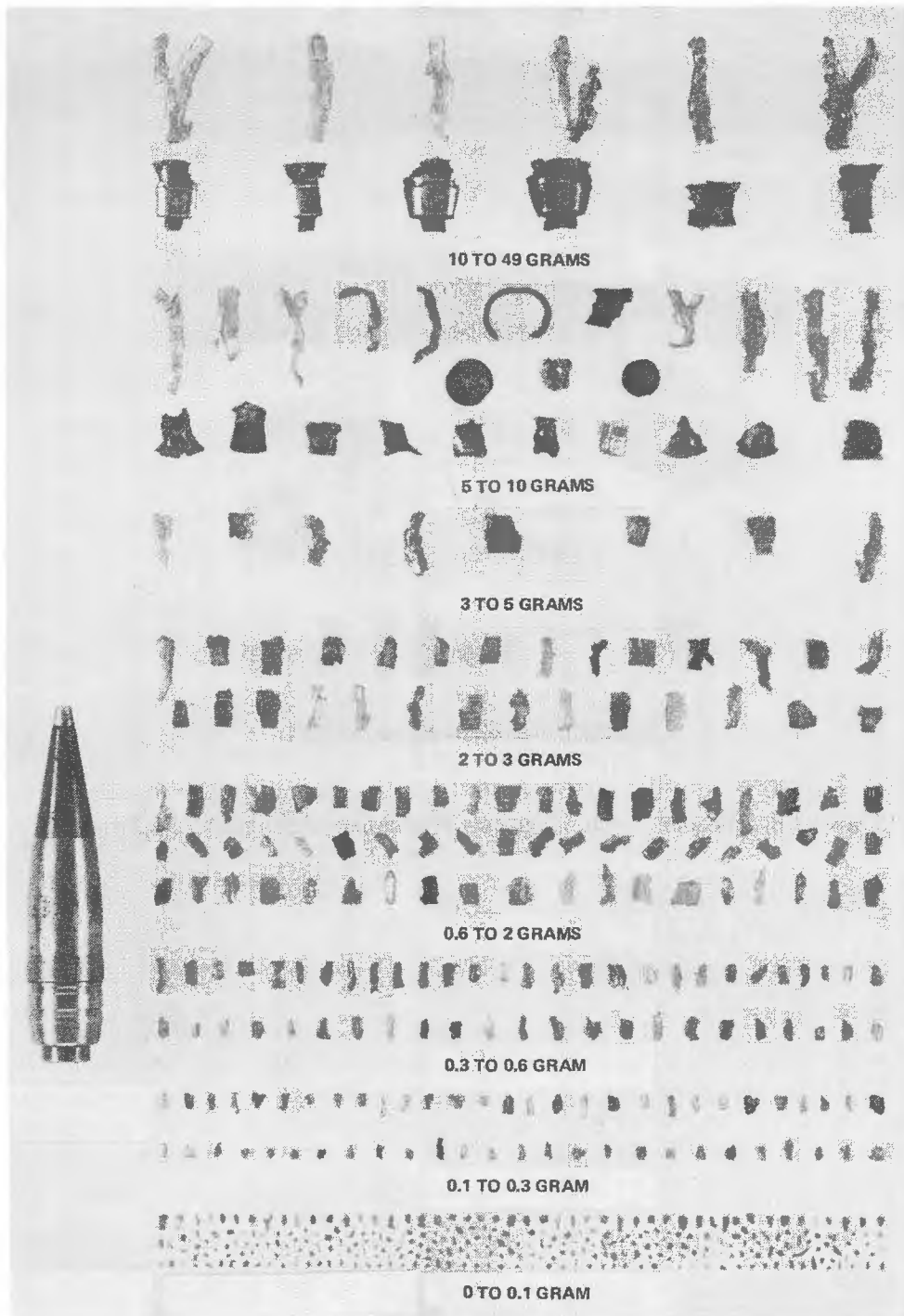
Figure 1-2. Soviet 27-mm Fragments From Model OR-167 Frag-T Projectile
