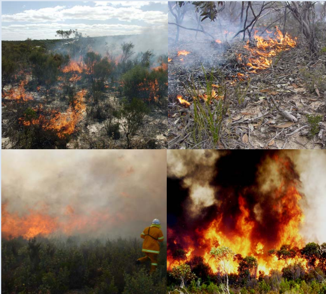
Range in fire behaviour observed in mallee-heath experimental fires. Top-left: Break-up of flame front in discontinuous heath vegetation under marginal burning conditions; Top-right: Marginal propagation in mallee litter; Bottom-left: Moderate intensity, fast spreading fire in heath fuels; Bottom-right: High intensity experimental fire in mallee-heath fuels (clump height 2.5 - 3 m).
