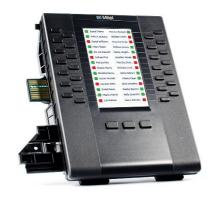
The Mitel M685 features a color LCD screen and 28 programmable keys, with the ability to scroll through three pages of programmed entries.
