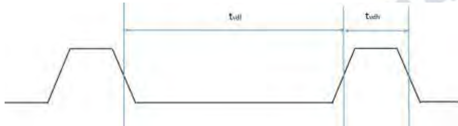
Figure 6.5-1: Tearing effect output signal mode 1
