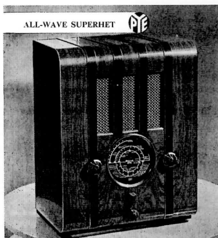
MODEL QAC 5. Six-valve (including rectifier) superhet for A.C. mains. 100-250 volts, 25-100 cycles. Consumption 95 watts. Five wavebands: 6.5-10 (including television sound), 11-28.6, 24-66.7, 200-565, 880-2,000 metres. Quiet delayed A.V.C. Planetary coil units. Flywheel tuning. Four-position selectivity and tone control. Output 7 watts. Dimensions: 21" high, 16½" wide, 10½" deep.
