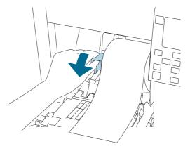
1 1 According to the paper width, open and/or close the platen shutters following the instructions on the label attached to the top surface of the printer.
