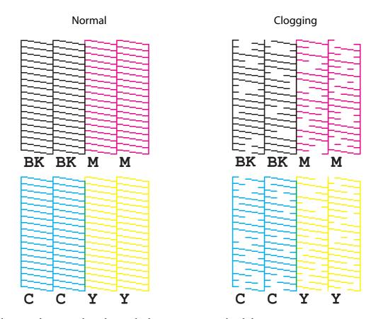
When the printed patterns show the nozzle clogging state, run a head cleaning.
