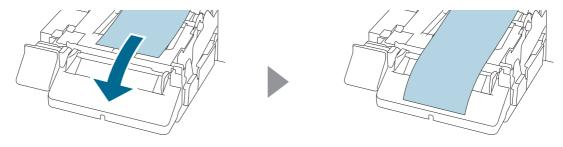
15 Hold down the paper by hand, and slide the paper ejection guides against the paper.
