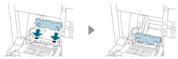
According to the paper width, open and/or close the platen shutters following the instructions on the label attached to the top surface of the printer.
