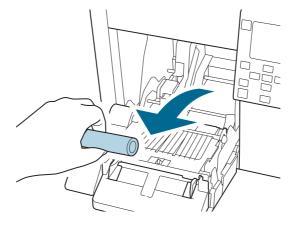
3 Attach the OT-WA34 by inserting it into the grooves inside the front cover.
