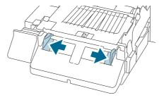
Raise the lock lever of the paper ejection guides until it clicks into place.
