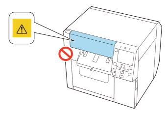
• To prevent fingers from being trapped, the lock mechanism is activated to stop the cover closing if the unit is raised up from the installation surface. When using the product, install it on a level surface.
