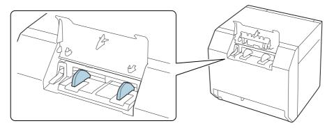
Remove any adhesive that has adhered to the inner surface of the paper feed guide.
