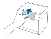
12 Raise the lock lever of the fanfold paper guides.
