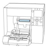
Remove any adhesive that has adhered to the inner surface of the paper guides.
