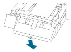
13 Slide the paper ejection guides outward.
