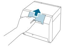
4 Remove the paper feed guide, and then close the rear cover.
