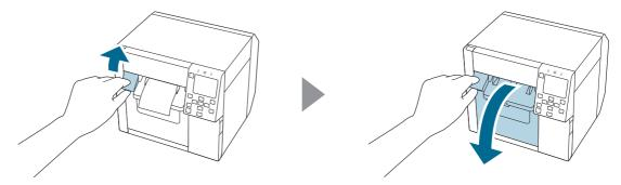
If the paper feed guide has been attached, remove it.
