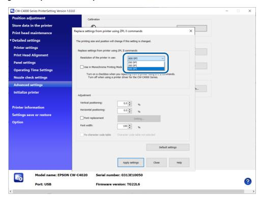
4 Select the checkbox for [Use in Monochrome Printing Mode] to print only in black and white and not print in color after replacing from the ZPL II compatible monochrome printer.
