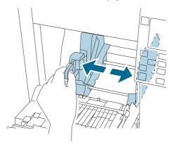
6 Lower the lock lever of the roll paper guides.
