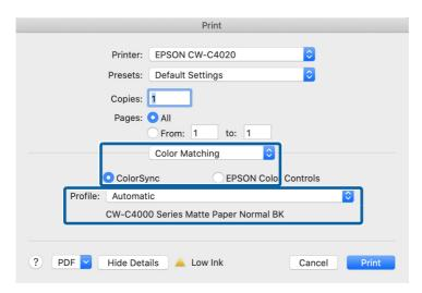
The default profile setting is [Automatic] which automatically selects an ICC profile provided by Epson.
