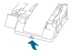
17 Pull out the leading edge of the roll paper, and then close the front cover.
