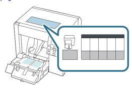
**7** Lower the lock lever of the paper ejection guides.
