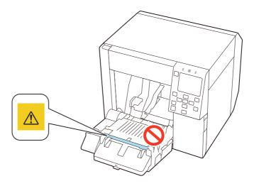
• Do not touch the movable blade of the auto cutter with a hand. Doing so may cause injury. As the label is affixed to the back of the auto cutter unit, it can be checked when the unit is removed.
