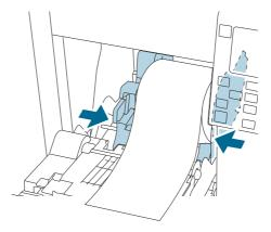
10 Lower the lock lever of the roll paper guides.
