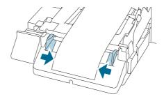
16 Raise the lock lever of the paper ejection guides until it clicks into place.
