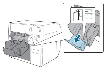
**A** Push in lever at the bottom right of the tray to lock it in place.
