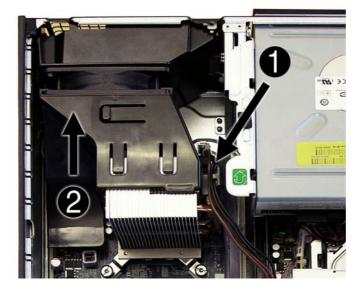
To install the baffle, reverse the removal procedure.
