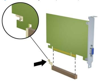
Figure 9-11 Removing a PCI Express x16 Expansion Card
