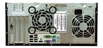
5. Lift the fan out of the chassis.
