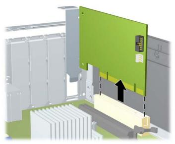
Figure 9-10 Removing a Standard PCI Expansion Card
