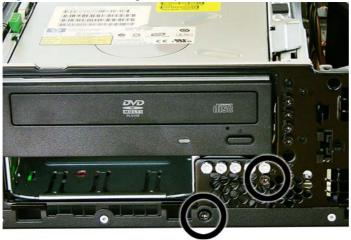
7. Lift the speaker from the inside of the chassis to remove it.
