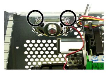
To replace the speaker, reverse the removal procedures.
