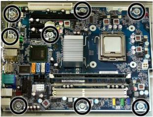
**13.** Lift up the front of the system board, and then pull the system board forward, up, and out of the chassis.
