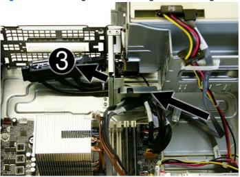
Figure 9-49 Guiding the wires through the drive cage
