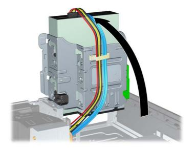
Rotate the power supply to its upright position. The hard drive is located beneath the power supply.
