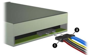
Figure 8-16 Disconnecting the Optical Drive Cables
