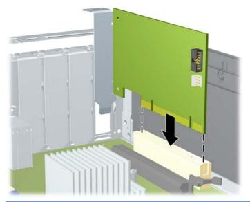
Figure 9-12 Installing an Expansion Card
