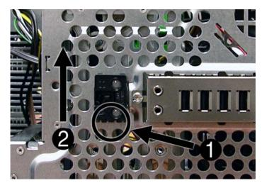
6. Pull the assembly away from the chassis while threading the cable through the hole in front of the chassis.
