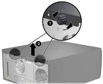
Figure 8-2 Removing the Computer Access Panel
