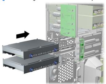
Figure 8-28 Sliding a Hard Drive into the Drive Bay
