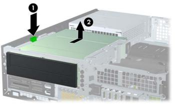
Figure 9-21 Removing the 5.25-inch Drive
