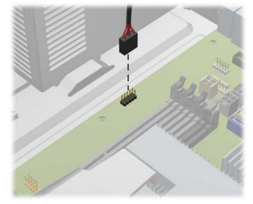
Figure 8-23 Connecting the Media Card Reader USB Cable
