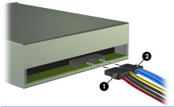
Figure 8-22 Connecting the Optical Drive Cables
