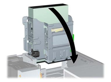
7. Press down on the green drive retainer button located on the left side of the drive to disengage the drive from the drive cage (1). While pressing the drive retainer button, slide the drive back until it stops, then lift it up and out of the drive cage (2).
