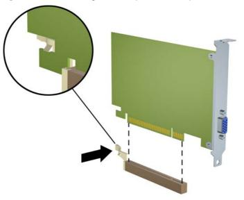
Figure 8-11 Removing a PCI Express x16 Expansion Card
