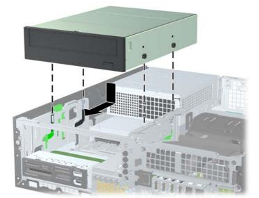
Figure 9-23 Installing the Optical Drive
