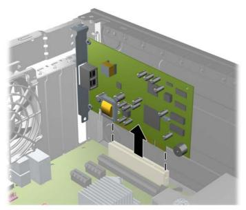
Figure 8-10 Removing a Standard PCI Expansion Card
