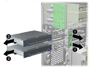
5. Remove the four guide screws (two on each side) from the old drive. You will need these screws to install a new drive.
