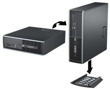
Figure 9-66 Changing from Desktop to Tower Orientation
