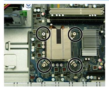
4. Remove the heat sink from the processor.
