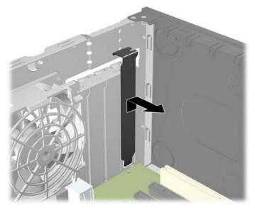
**b.** If you are removing a standard PCI card or PCI Express x1 card, hold the card at each end, and carefully rock it back and forth until the connectors pull free from the socket. Pull the expansion card straight up from the socket then away from the inside of the chassis to release it from the chassis frame. Be sure not to scrape the card against the other components.
