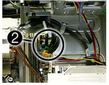
8. While holding the body of the assembly, pull the assembly away from the front of the chassis while guiding the cables through the hole in the drive cage (3).
