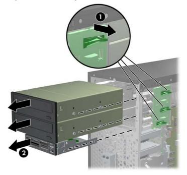
6. Remove the four guide screws (two on each side) from the old drive. You will need these screws to install a new drive.
