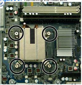
Figure 9-51 Removing the heat sink
