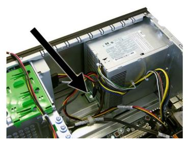
6. Slide the power supply toward the front of the computer, rotate toward the fan so the power supply clears the lip on the top of the chassis, and then lift the power supply out of the chassis.
