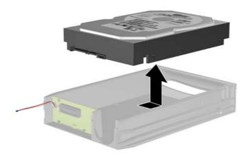
6. Place the new hard drive in the carrier then slide the hard drive back so that it seats in the SATA connector on the carrier's circuit board. Be sure the connector on the hard drive is pressed all the way into the connector on the carrier's circuit board.
