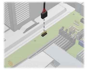
Figure 8-18 Disconnecting the Media Card Reader 1394 Cable
