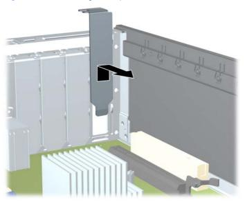
Figure 9-9 Removing an Expansion Slot Cover
