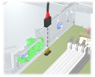
Figure 9-28 Disconnecting the Media Card Reader 1394 Cable
