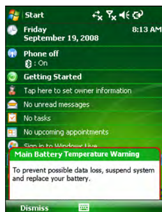
Figure 2-9 Main Battery Temperature Warning Dialog Box
