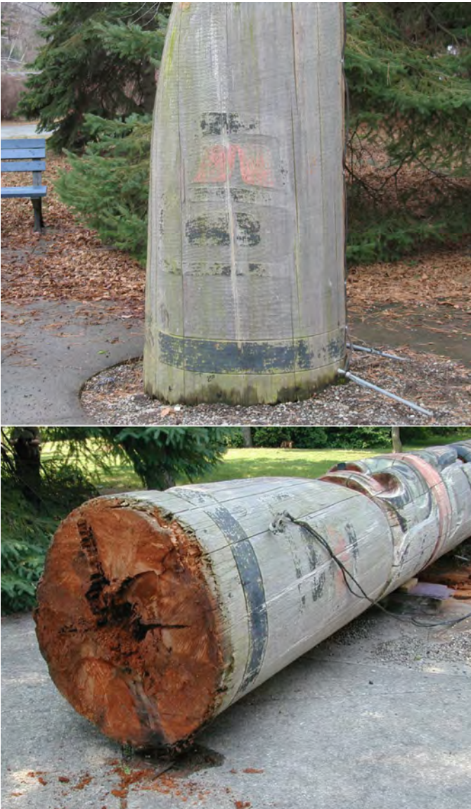
Figure 1. The Hunt Family Pole in Montreal, 2006. Although apparently in excellent condition (top), only 3 to 5 cm of good perimeter wood remained around a rotten core and central void (bottom).
