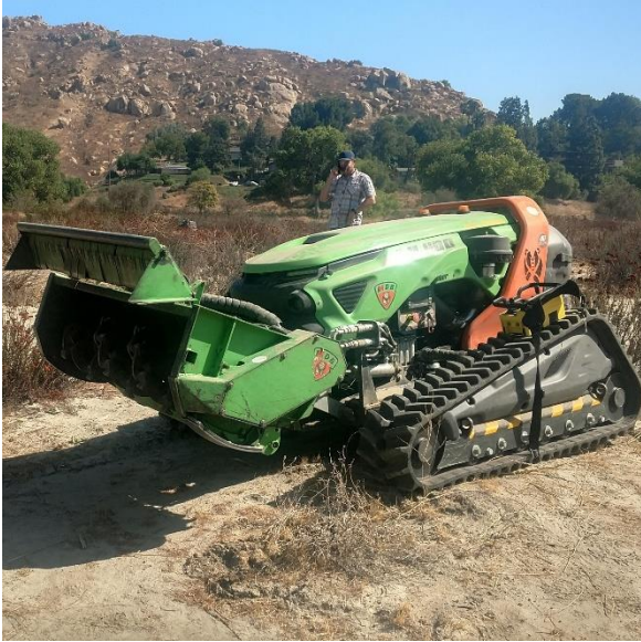
Flail mowers can be used on heavy brush. Left: Remote-control flail mower. Photo credit: Jutta Burger. Right: Mature French broom successfully removed with flail mower. Photo credit: Pamela Beitz.
