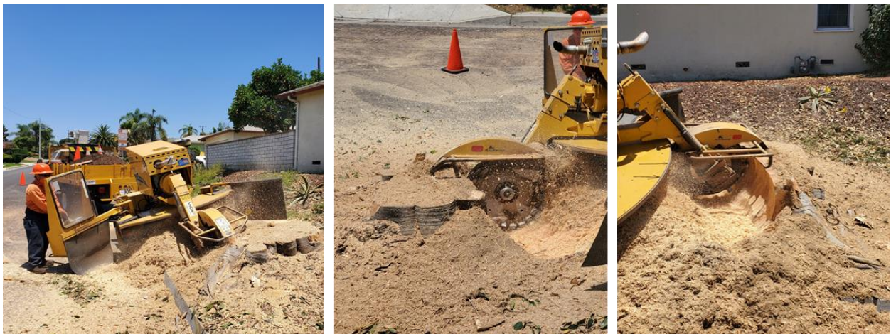
Stump grinding a residential tree ( Ficus elastica ). Photo credit: Dane Jensen, West Coast Arborists, Inc.
