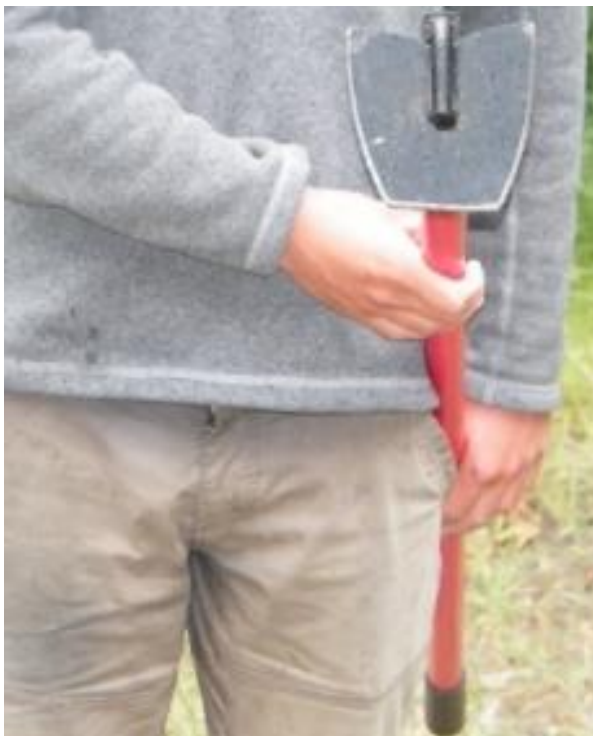
Two modified tools for removing artichoke thistle rosettes. Left: Triangle hoe with tip cut off and edge sharpened. Photo credit: Sandy DeSimone. Right: Shovel bent, welded, and edge sharpened. Photo credit: Claire F. Meyler.
