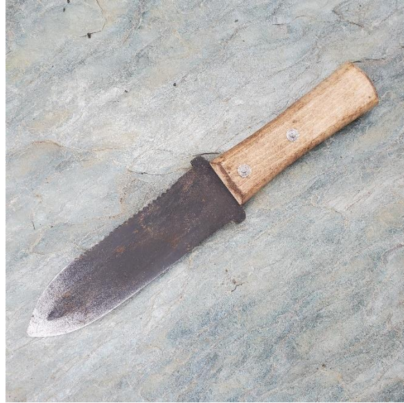
Common tools used for whole plant removal of smaller weeds. Left: Hand trowel and forked weeder. Right: Soil knife or hori-hori. Photo credit, both images: Jutta Burger.
