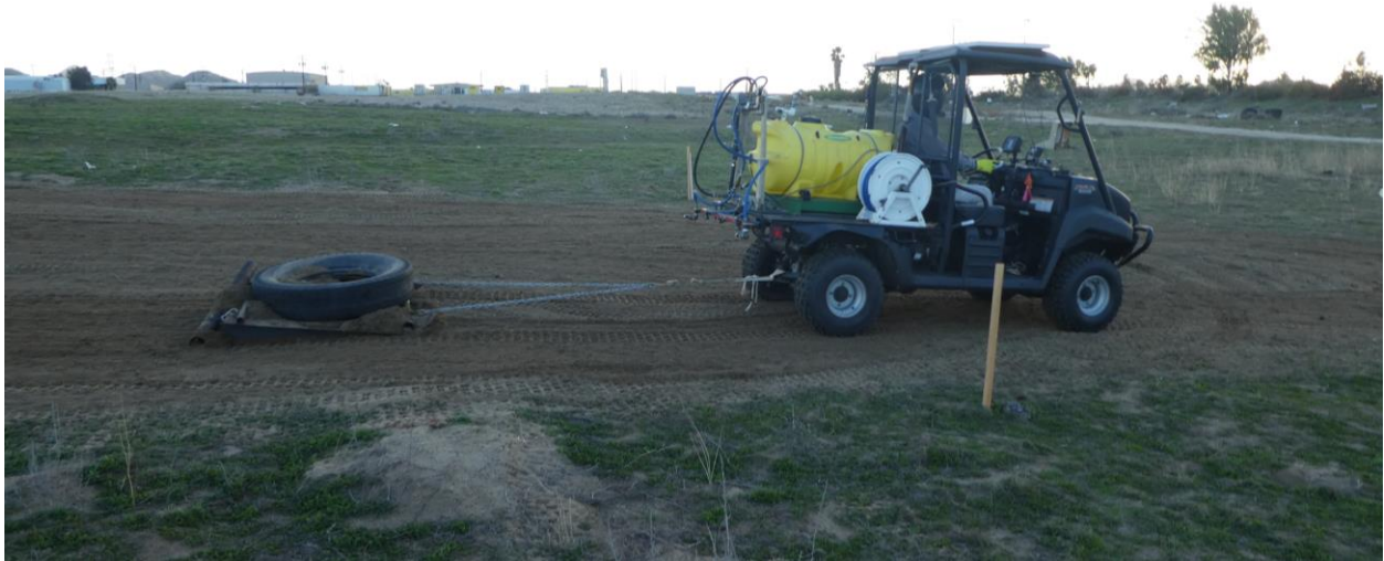
A 4x4 UTV pulling a modified harrow weighted down by an old tire as a winter seedbed treatment for a shrub restoration plot. Note that there is low residual plant cover and weeds are small. Photo credit: Ryan Lawler.
