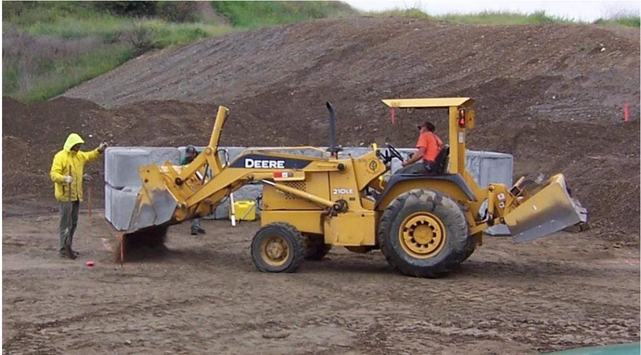
Skip loader with articulating bucket on front and box scraper on back. Photo credit: Rodney Smith.
