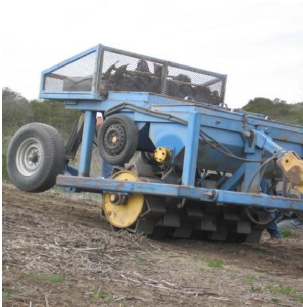
After prepping site through grow-and-kill with herbicide and mowing, this site in Irvine was replanted. Left: Seed imprinter to improve seed-soil contact. Photo credit: Megan Lulow. Right: Seeding needlegrass with a wildland seeder. Photo credit: Lars Higdon.
