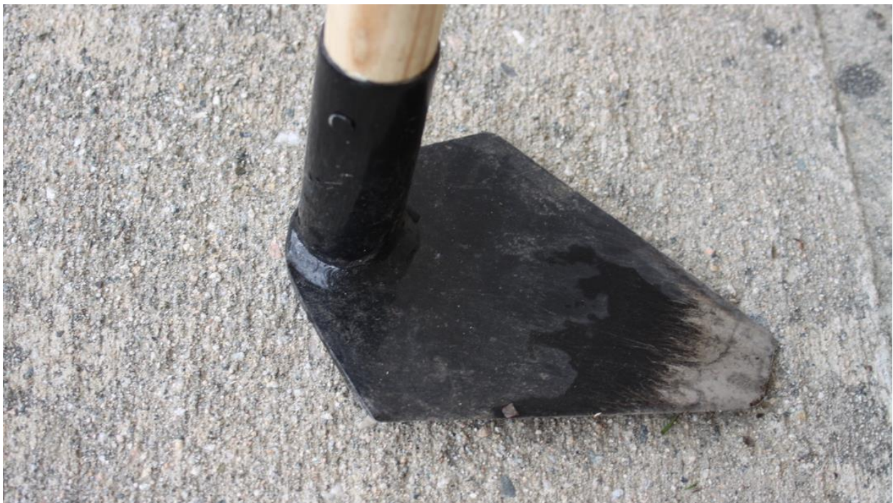
A triangle-shaped grub hoe, with a blade tapering from 5 inches at the widest to 1.25 inches wide at the tip. Photo: Christopher McDonald.
