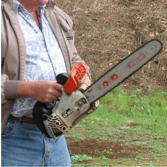
Left: Fourteen-inch bar gas-powered chainsaw, the most commonly-used size range for woody invasive plant management; held here for scale, and not to be used without proper PPE. Photo credit: Cal-IPC archives. Right: Mid/large-sized gas-powered chainsaw for larger trees. Photo credit: Tom Getts.
