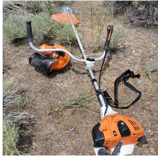
Left: Bump-head line trimmer attachment. Right: Heavy-duty brush cutter with metal circular blade, U-shaped handles, and harness. Photo credit: Tom Getts.
