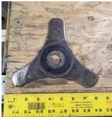
Three weed trimmer head attachments for tougher vegetation. Left: Heavy-duty fixed-line trimmer head. Photo credit: Shawn Thorin. Center: Tri-bladed brush cutter blade. Photo credit: Shawn Thorin. Right: Circular brush cutter blade (for woody material). Photo credit: Tom Getts.
