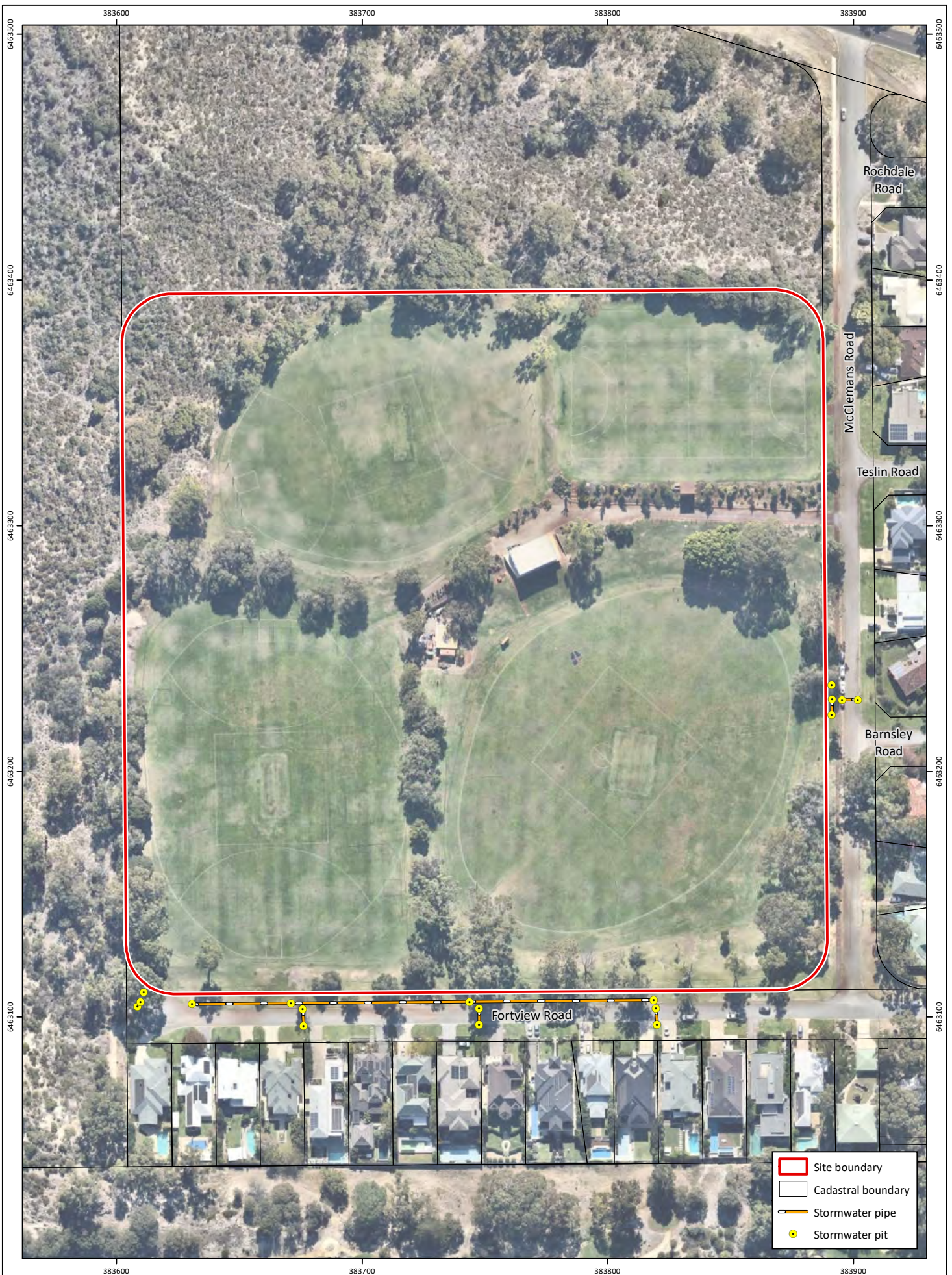
Figure 4: Existing Stormwater Infrastructure
