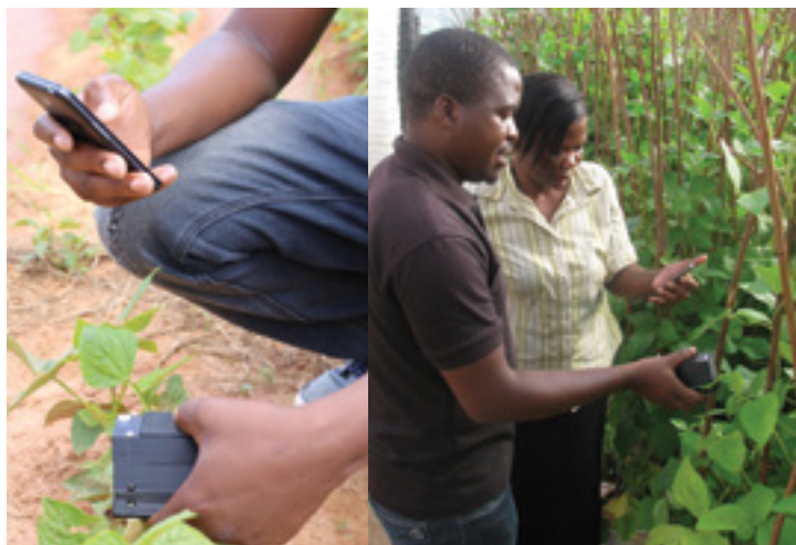
Taking photosynthesis readings using the MultiSpec and PhotosynQ—in the field and under controlled conditions.
