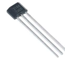
HX3144UA (Container Revolution Counter Sensor)
