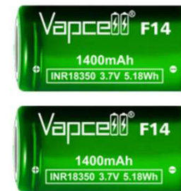
Vapcell 18350 F14 (Payload Battery)
