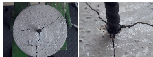
Figure 7: Splitting failure at UHPC | photos: Frank Schladitz
