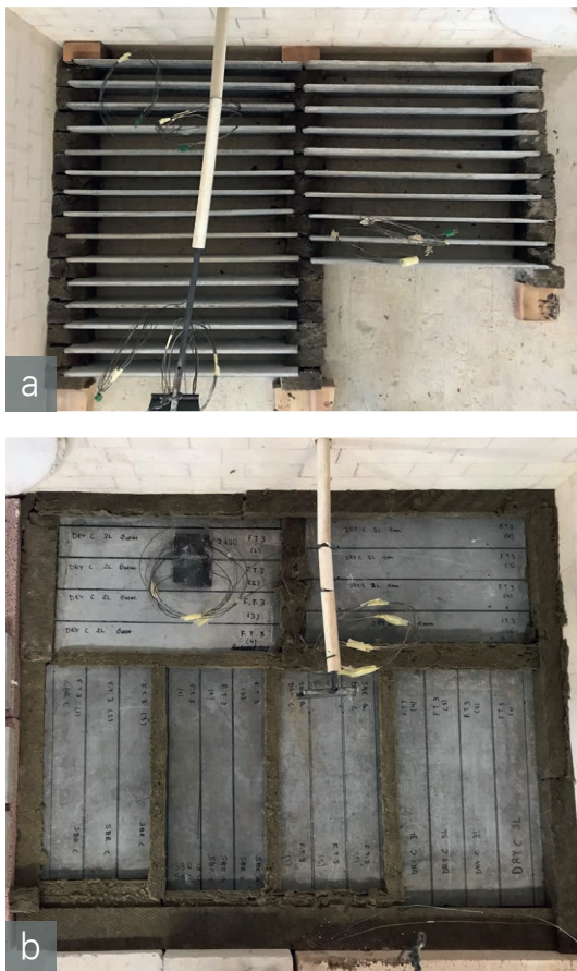
Figure 2: (a) positioning of tension specimens in the furnace; (b) positioning of flexure specimens in the furnace | photos: Panagiotis Kapsalis
