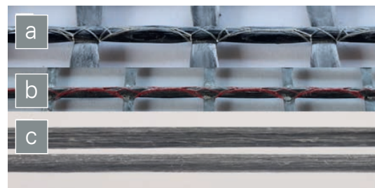
Figure 1: Carbon reinforcements under investigation: a) Epoxy (EP), b) Acrylic based polymer (ACR) and c) two mineral-bonded carbon reinforcements (MIN-60 and MIN-80) | photos: Kai Schneider
