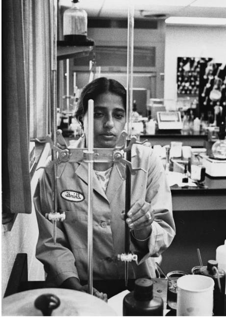
*Employee Shindi Mahal, lab technician, tests the sulphur dioxide content of corn syrup at a corn milling plant in Dayton, Ohio, 1973.*
