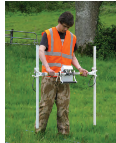
Illus. 2 - Archaeological geophysical survey can take many forms. This is an example of Fluxgate Magnetometry, which measures minute variations in the earth's magnetic field which can be interpreted to indicate buried archaeological features.
