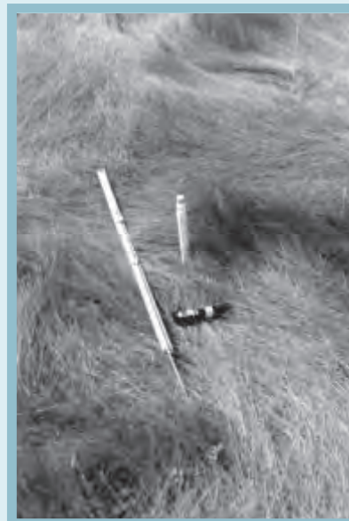
Water table salinity monitoring well, with refractometer for measuring salinity and modified meter stick to measure water level
