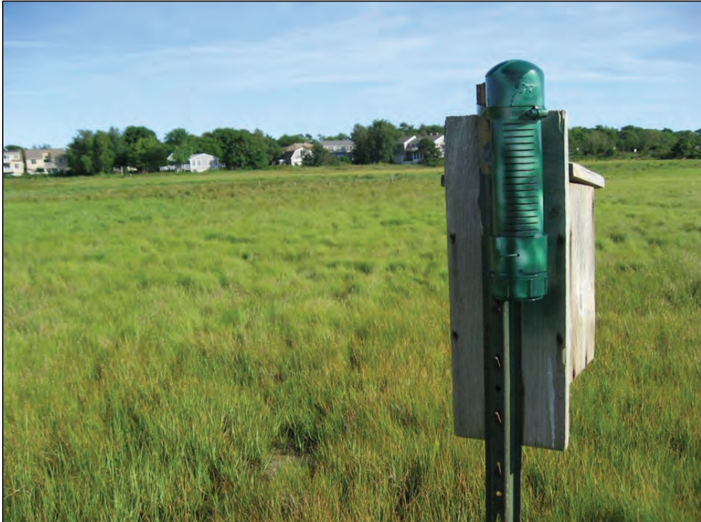
Figure C 3. Barometric sensor attached to bird nesting box (Rachel Carson National Wildlife Refuge, Maine).
