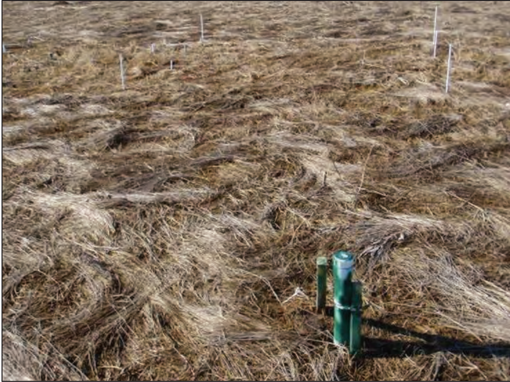
Figure C 2. Water level sensor in a wetland (Rachel Carson National Wildlife Refuge, Maine).
