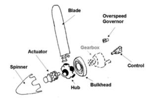
Figure 1 Major Propeller Components
