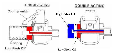
Figure 3 Single- and double-acting systems
