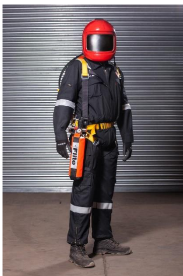
Figure 6: Operator with integral helmet and full breathing apparatus. The picture on the right shows the top of a reactor with fall arrest tripod.
