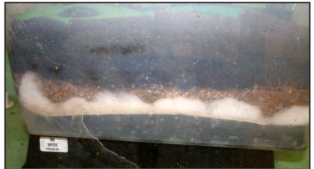
Step 3: Layers of foam, filter floss and gravel to create biological media
