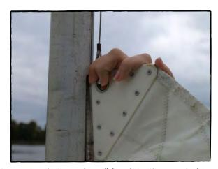
Photo 22, Feed the main sail luff into the mast slot
