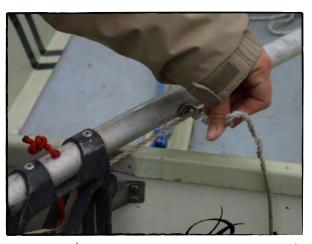
Photo 37, Attach the rudder uphaul
