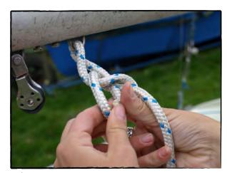
Photo 31, attach the mainsheet to the boom
