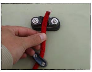
Photo 13, Pass the jib sheets through the jammers
