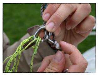
Photo 9, Attach the jib to the halyard
