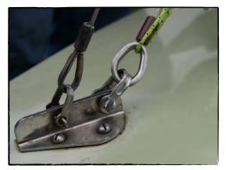
Photo 8, Attach the jib to the chainplate
