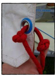
Photo 12, attach the jib sheet
