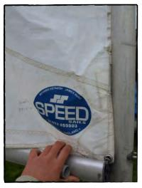
Photo 24, boom onto gooseneck
