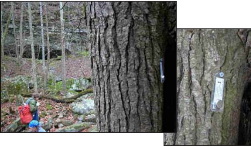
Figure 10: iButton units mounted to trees external to the cave monitor the local weather.
