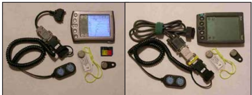
Figure 4, right: One of the lessons learned was to have a backup PDA on long trips in case a defective cable or iButton unit caused a problem with in-cave missioning. This Palm IIIxe with a monochrome screen required a different serial adapter for the older PDA unit. It connects to the same iButton Blue Dot adapter and used two Alkaline AAA batteries.
