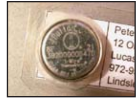
Figure 2: The iButton case looks like a large watch battery. They were mounted on tags for the experiments in the caves.
