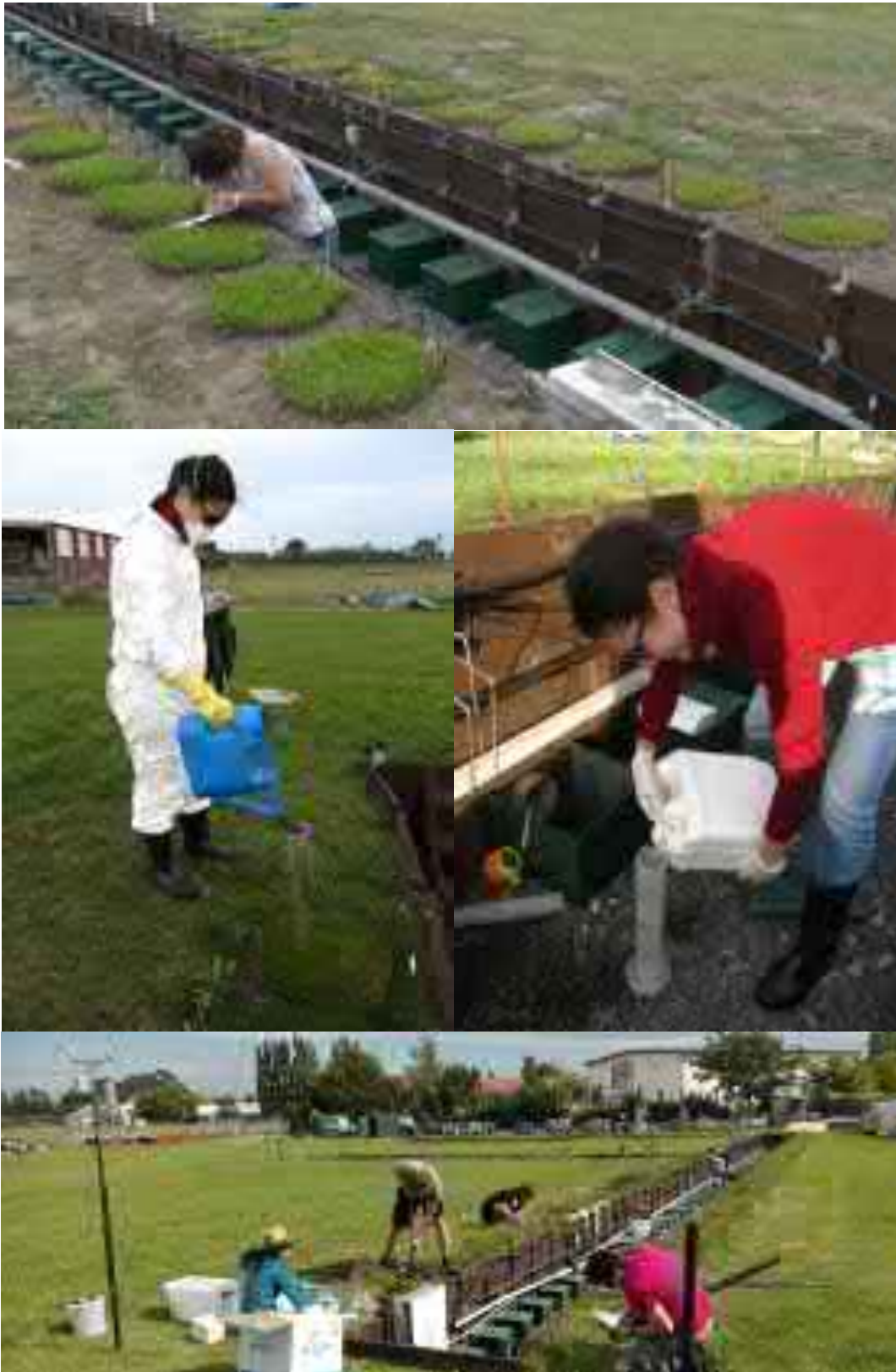
Fig. 3. Top: The installed lysimeters showing the six Pawson silt loam soil cores (front-left) and the 12 Barry's soil cores (rear-right). Centre left: Effluent application. Centre right: Drainage collection. Bottom: Destructive sampling of the lysimeters at the conclusion of the experiment. 16 th of November, 2016.
