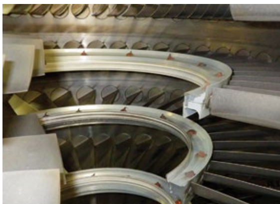
16. LM2500 compressor looks new after having operated for more than 22,000 hours at base load with no water washes
