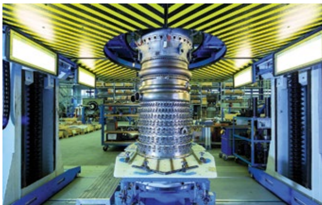
9-11. Efficient shop workflows and highly developed processes at MTU assure short turnaround times. Technician completes overhaul of an LM6000 in Fig 9 (above), build-up stand for an LM engine is in Fig 10 (left), and the teardown/re-assembly line at Ludwigsfelde is captured in Fig 11 (below)
