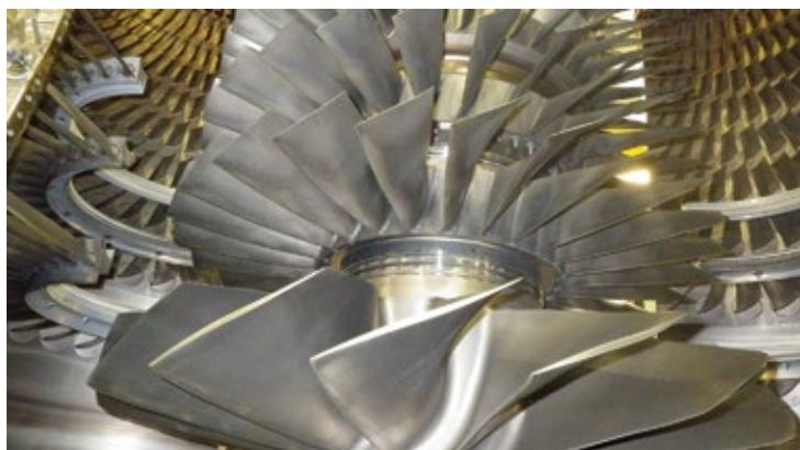
16. LM2500 compressor looks new after having operated for more than 22,000 hours at base load with no water washes
