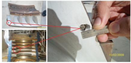
1. Plug weld liberated from an R2 strongback diaphragm and traveled downstream in the compressor, damaging many blades in the process
