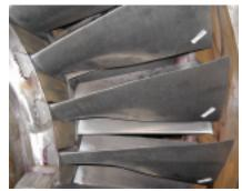
2. Stake marks indicate this is the third set of R0 blades. The next change-out will require the OEM to install its "Biscuit" mod before installing the blades
