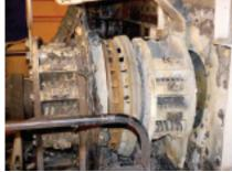
**19. Catastrophic failure** was caused by a flashover between polarities
