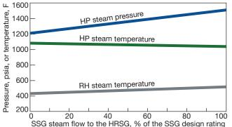
**20. Steam conditions** at the steam turbine's HP and IP inlets show little variation, except for HP steam pressure, over the full range of SSG outputs
