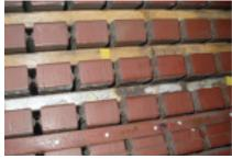
7. Advanced partial discharge activity is in evidence on bar surface
