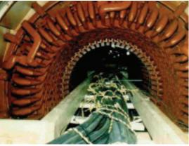
**24. Excitation coil** is arranged for high-flux test
