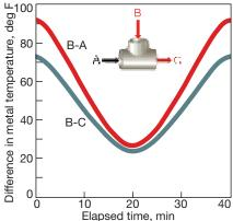
**22. Temperature variation** in mixingtee metal temperature during solar transient suggests a fatigue analysis C (HP superheater inlet) goes from 627F to 596F in the first 20 minutes of the cycle.
