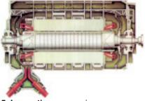
**5. Inspection access** in an assembled generator is limited as the cross section of a typical unit attests
