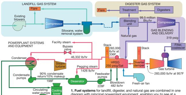
diagram with principal powerplant equipment, enabling you to see at a glance how the new cogeneration plant is arranged
