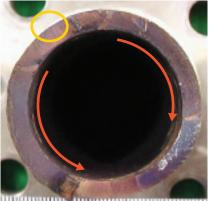
**20. Analysis of fracture surface** revealed striations characteristic of HCF along the red arrows. Starting point of the cracks appeared to be in the yellow circle at the back ends of the arrows (left)
