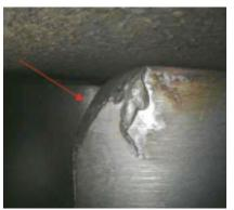
6, 7. R2 blade trailing-edge (left) and S2 vane leading-edge (right) clash indications typically look like this when viewed through a borescope
