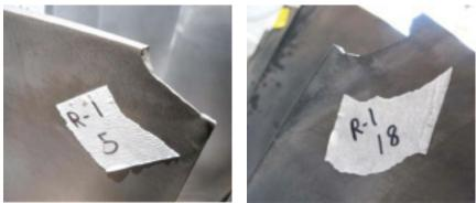
**1. Classic tip crack** is shown at the left with crack initiation about 2 in. from the leading edge. Impact caused the damage at the right
