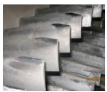
**5. Cropped S2 leading edge** during an outage. Technicians took precise measurements of the damaged area on each vane then cropped the worst airfoil and cut back the entire row to the same point
