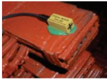
**1. Stator end-winding vibration** sensor is mounted on a winding series connection
