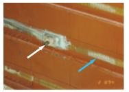
4. Flux probe (white arrow) is highly reliable and can determine the precise coil where a short exists. The green arrow points to seven holes in the wedge for measuring radial spring compression height. which is indicative of the wedg-
