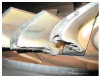
**12. Bucket damage** at the leading edge and coating detachment resulted from forward migration of the airfoils
