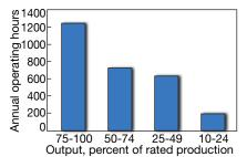
Output, percent of rated production **19. Annual capacity factor** of the solar steam system is 32% for a typical year with 2810 operating hours keep mirrors clean and maintain the thermal fluid system (often referred to as heat-transfer fluid, HTF) that transports heat from the solar field to the SSG.
