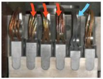
**25. Lead discoloration** (red arrows) and selective action (blue arrow) are in evidence above. Latter is no longer capable of carrying current
