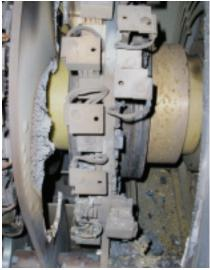
**26. Aftermath of a flashover.** Brushbox carbon deposits compromised brush-to-ring connections and caused arcing, which escalated into a serious fire
