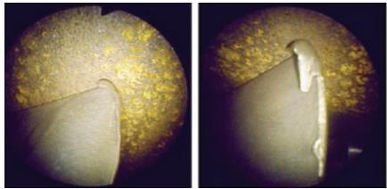
**8. Smeared and rolled metal** on adjacent stator vanes (damage area on vane at left,  $1 \times 0.25$  in.; at right,  $1 \times 0.375$  in.) proved clashing was increasing in severity since its discovery a year earlier
