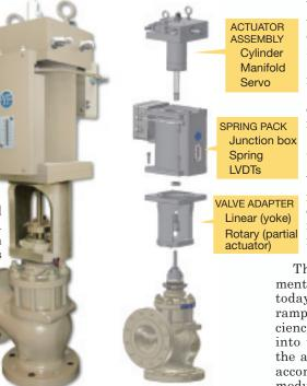
**30. New generation of modular,** ruggedized valve actuators under development offers design simplicity, high reliability, field serviceability
