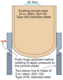
**10. Redesigned guide sleeve** for piccolo pipes is easy to make and doesn't require cutting the existing pipes
