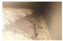
8. Spark damage caused by vibration is seen in ventilation duct through a borescope
