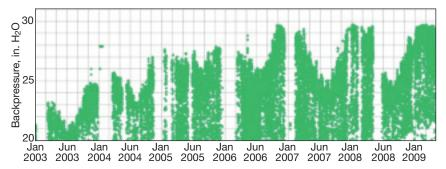
**6. HRSG backpressure** over time illustrates seasonal variations—valleys in summer, peaks in winter. Boiler limit is 30 in.  $H_2O$ , forcing operators to manually limit gas flow through the HRSG on occasion by changing position of compressor inlet guide vanes
