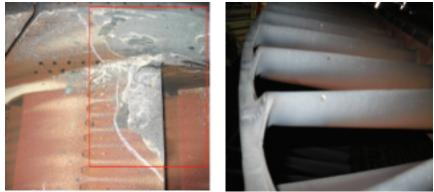
**14, 15. Fallout** from the first-stage bucket migration issue includes damage to first-stage vanes and second- and third-stage buckets
