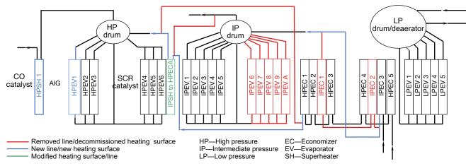
4. Heat-recovery steam generator, which supplies STIG and NO<sub>x</sub> steam to the gas turbine required a redesign effort, some new components, and modification of others to accommodate the change in engines from LM5000 STIG 120 to LM6000-PC CDP
