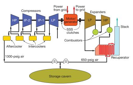
**13. First-generation CAES** is characterized by a single train of air-cavern charging compressors and external combustors for the expanders
