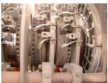
**18. Arc damaged rings** on only one polarity of brush-holder rigging
