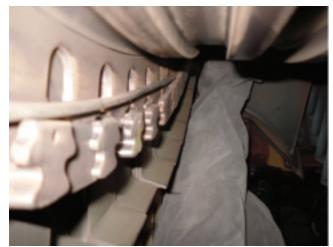
**13. Lockwire** is clearly out of the groove provided, compromising its ability to hold buckets in position
