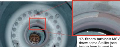
**17. Steam turbine's** MSV threw some Stellite (see insert) from its seat in November 2006, damaging HP nozzles and blades (see Figs 18 and 19)
