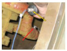
**22. Bump tests** are suggested for in-service stator endwindings experiencing vibration problems. Yellow arrow points to impulse hammer, red to pick-up
