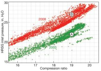
**5. Historic data** show a nominal increase in HRSG inlet pressure of 5 in.  $H_2O$  (point A to point B) over a five-year period because of fouling
