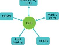
31. CDM system continuously monitors combustion dynamics and relays this information to the DCS, which monitors emissions and sends data to the auto-tuning PLC. The PLC determines when adjustments are necessary and automatically tunes the turbine to the operator's optimization goals.
