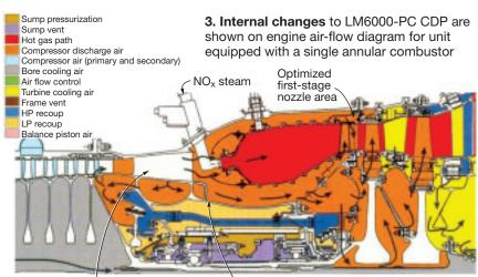
STIG steam injected into existing compressor discharge bleed ports
