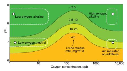
**2-8. The basics of stator water chemistry:** High-purity water is a good insulator, copper in water is prone to oxidation, the rate of oxide release depends on pH and oxygen concentration
