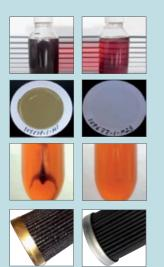
**Before** & **after** installation of a CJC™ Varnish Removal Unit VRU
