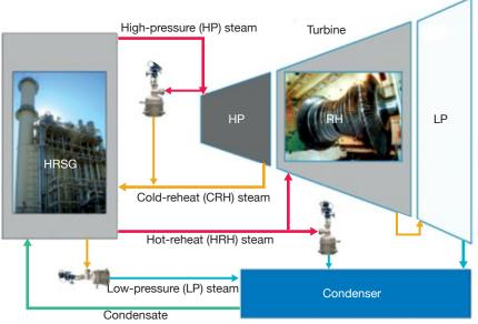
6. Severe service valve installed in the HRH bypass system at Australia's coalfired Millmerran Power Station (left)
