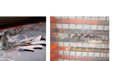
**4-2. Failure to ground** caused by the fracture of a stator conductor is not rare. Winding and core damage attributed to a burned open bar in a slot is shown at left and right, respectively
