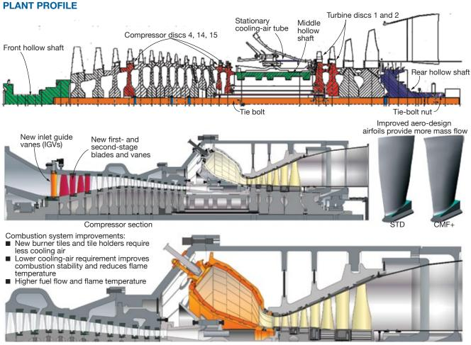
2. Three major elements of the gas turbine/generator refurbishment were replacement of parts for life extension (top); modification of the compressor for higher mass flow (center), including I&C mods for surge control and new IGV position sensor; and combustor improvements to increase output and provide better flame stability (bottom)
