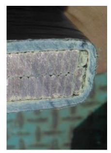
of **1-11. Voids visible** at the bottom of the bare bar were caused by internal PD COMBINED CYCLE JOURNAL. Third Quarter 2015
