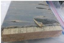
**1-9. Investigators identified severe** internal and external partial-discharge damage on high-voltage bars. Note damage to surface tapes and grounding paint
