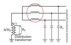
**4-1. Stator windings** of large generators typically are wye-connected and high-impedence-grounded through a distribution transformer
