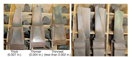
**1. Effect of poor coating thickness** appears visually (and dramatically) after a baseload HGP period of operation at 2035F. Coating was non-OEM "GT33 equivalent"
