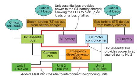
**Redesign of the distribution system** at Athens corrected an electrical service deficiency. The thick color lines trace the unit essential bus and cross-tie additions that have greatly improved operating flexibility and speed of recovery from emergency conditions
