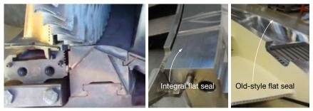
**4. New integral seal** is much more difficult to repair correctly, even for normal wear, than the old style replaceable seal
