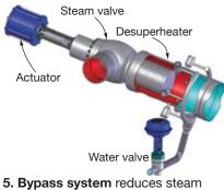
**5. Bypass system** reduces steam pressure and temperature before it enters the turbine
