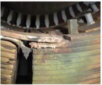
**3-1. Failure modes** discussed by Moore included the pole-to-pole crossover failure shown here
