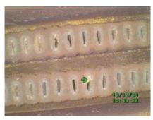
2-7. Effects of restricted flow caused by oxide formation are in evidence here
