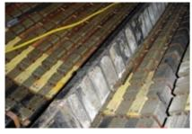
**2-4. Winding deterioration** was caused by bar vibration in the slot (vibration sparking)
