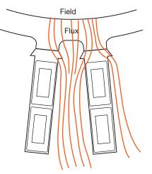
**1-12. Magnetic flux** moves quickly into tooth iron after crossing the air gap
