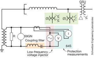
$R_G$ . This relay system leaves undetected grounds in the low-voltage end of the winding. Examples are shown in Fig 4-2. Four such recent failures in a two-year period involved repair costs of close to \$500 million. Full winding protection can be obtained by using an injection relay, 64S. But **4-3. Voltageinjection** ground protection can be functional when the generator is shut down (standstill or turning gear), during startup, and at speed offline and online
