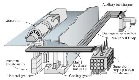
**1. Electrical energy** produced by the generator is moved via isophase bus to transformers that boost voltage for export to the grid or for in-plant use
