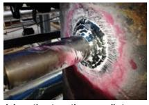
**4. Insertion-type thermowells** in SA106B carbon-steel piping rely on an Inconel weld filler
