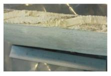
**1-10. Total destruction** of internal insulating materials is in evidence: Cross-over putty is completely eaten away and the strand insulation has been attacked
