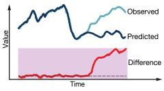
Advanced APR techniques, which detect the difference between actual (observed) and expected (predicted) trends in machine health and performance, are being integrated directly into the Ovation control platform and pilot tested at key customer sites
