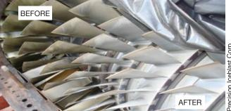
4. Compressor blade cleaning is a common ice applica-
