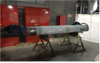
2. New HP bypass desuperheater has welds 10 ft farther downstream and includes a liner
