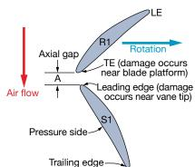
Axial gap (A) at R1 root: more than 0.600 in. Axial gap (A) at R1 tip: About twice gap at root the Hershey Lodge Convention Center in scenic Hershey, Pa.
