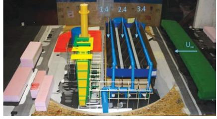
**17. A physical wind-tunnel model** was developed to advance the depth and breadth of the Caithness studies
