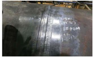
1. Desuperheater weld crack developed about 1 ft downstream of spray nozzles
