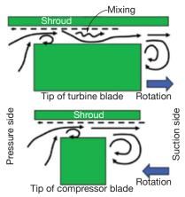
2. General leakage flow over the tips of turbine and compressor blades is basically the same
