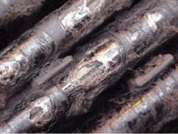
**12. Cleaning of generator stator** insulation requires care. Photo illustrates what can happen when blast pressure is too high
