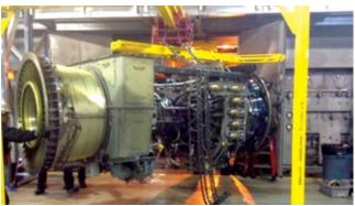
6. When rolling out the engine, the speaker's experience suggests having a person at each corner. The challenge at this site was the reduced clearance between grade and maximum engine height because the package was installed below grade
