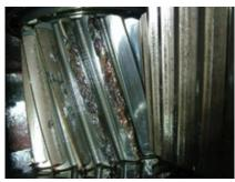
**11. Secondary pinion gear** damage suffered at Gateway Generating Station
