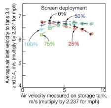
**15. Effects of wind speed** and windscreen deployment on the average air inlet velocity to fans 3.4 and 2.4 are illustrated in the chart. Note the positive effect of the screen at higher wind speeds and its negative effect at lower wind speeds. Breakeven is about 9 mph (4 m/s). Best results are achieved with 50% screen deployment (up to a wind velocity of 18 mph)
