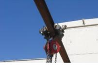
**1. Trolley system** with chain-fall hoist is used to move collector rings from oven to generator for installation
