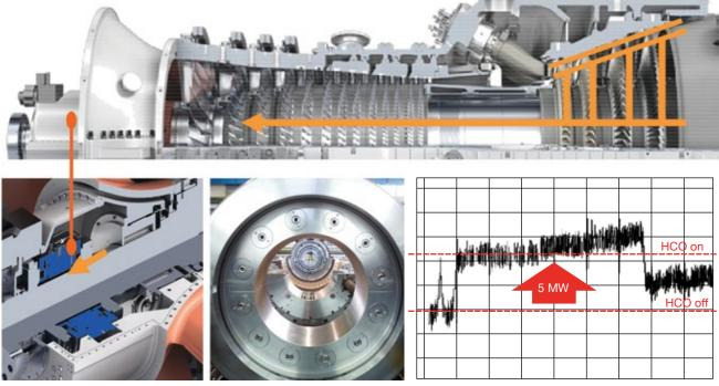
5. Hydraulic clearance optimization feature available on some Siemens gas turbines controls blade-tip clearances automatically by way of hydraulic pistons located behind the compressor thrust bearing
