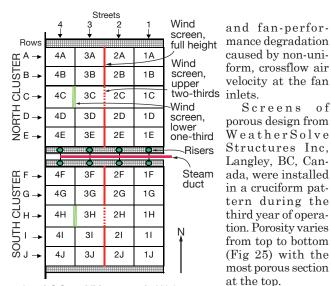
27. ACC at NV Energy's Walter M Higgins Generating Station has 40 cells, arranged as shown. Note location of screens and their different configurations
