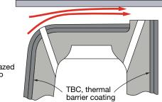
4. Computer modeling of tip leakage for turbine blade with conventional squealer tip is at left. Squealer tip design for original 501F firststage turbine blade (center) caused turbulence conducive to cap cracking and oxidation. Elimination of the squealer tip on one side of the 501F blade (right) smoothed out the flow, contributing to fewer repairs, longer life
