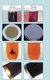
**Before** & **after** installation of a CJC™ Varnish Removal Unit VRU
