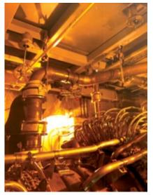
3. Air piping over the engine is rigged for bleed-valve removal
