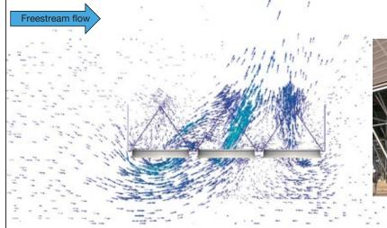
**1. Typical impact on ACC** of a 9-mph wind without windscreens installed
