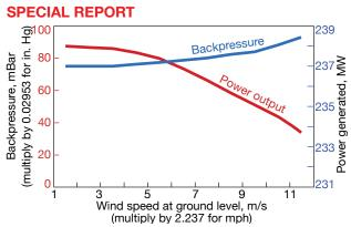
**7. ACC performance** falls off as wind speed increases. Results are for a 750-MW combined cycle operating at 50F ambient
