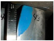
**3. Leading edge of stationary vane** was removed by contact with rotating blades
