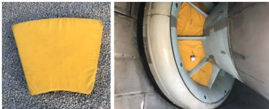
1. Custom-fitted inserts of high-density foam prevent air flow through the compressor and HRSGs when the gas turbine is on a weekend shutdown or longer
