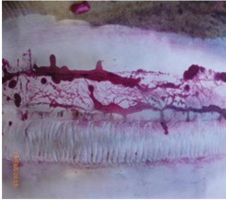
2. Stress corrosion cracking of austenitic stainless steel (Types 304 and 316) is easy to identify
