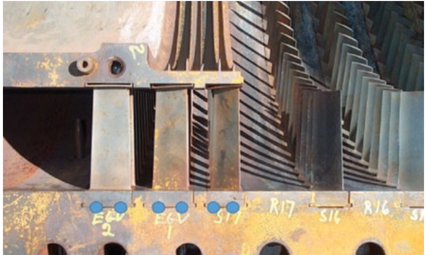
4. Coil pins absorb vibration that can cause fretting wear in rows S17, EGV1, and EGV2. They are inserted in holes drilled half into the vane ring segment base and half into the compressor discharge case
