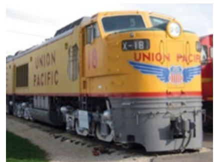
4. The Union Pacific had several locomotives powered by gas turbines in the 1950s
