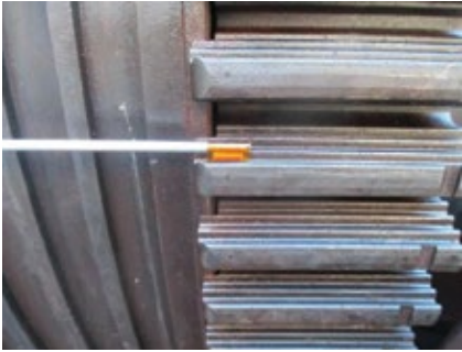
6. Eddy-current probe inspects dovetails for cracking, which could mean wheel replacement
