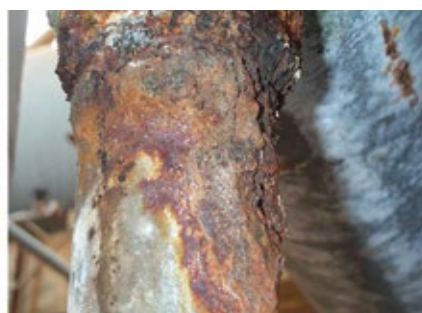
1. Atmospheric corrosion of carbon and low-alloy steel is hidden under insulation
