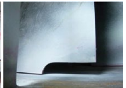
5. Rotor-blade radial tip crack like that at left can be removed in-situ (first and second stages) in one shift as shown in the photo at right. Were the crack allowed to propagate, a tip liberation might have occurred, with consequent downstream damage
