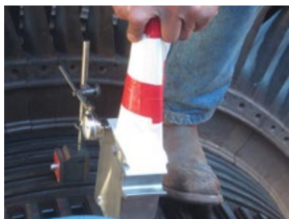
8. Bucket-rock measurements are taken with a dial indicator
