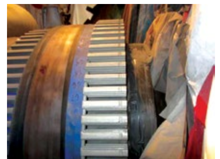
10. Dovetails after coating with nickel aluminide to mitigate bucket rock
