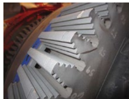
9. First-stage wheel after grit blasting
