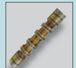
Varnish on valve spool
