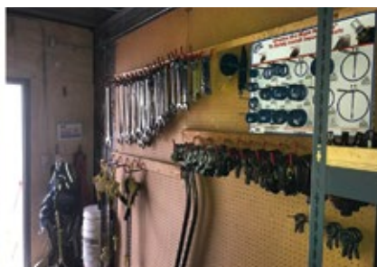
3. Portable crib for the tools recommended in GEK 107535 was designed by and for the O&M techs on the outage team
