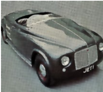
5. Jet One roadster is believed the first car powered by a gas turbine
