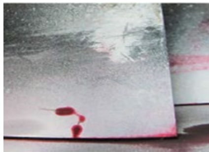
5. Rotor-blade radial tip crack like that at left can be removed in-situ (first and second stages) in one shift as shown in the photo at right. Were the crack allowed to propagate, a tip liberation might have occurred, with consequent downstream damage
