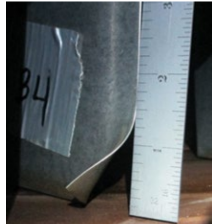
11. Bending of compressor blade reflects ice impact damage
