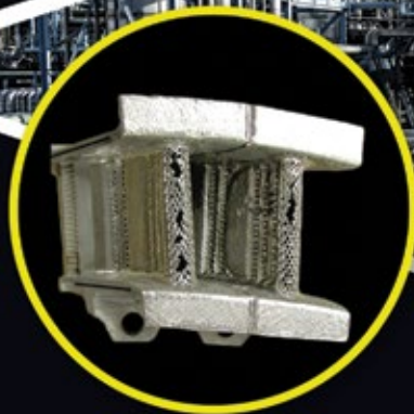
Damaged Vane (After Removal of Damaged Material)
