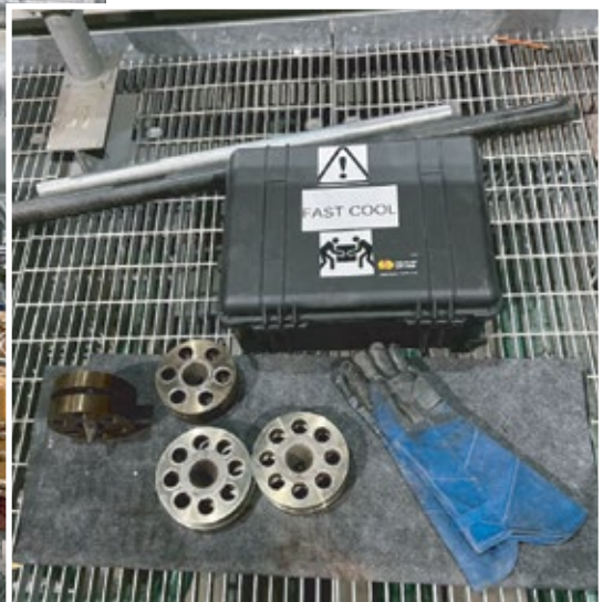
2. Toolbox is equipped to allow rapid replacement of blank flanges with the so-called fast-cool flanges shown
