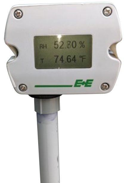
2. Sensor monitors both space temperature and humidity
