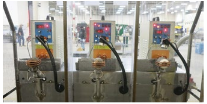
4. Tests of one new, one service-run, and one repaired fuel nozzle were conducted simultaneously to verify the viability of Liburdi's repair process
