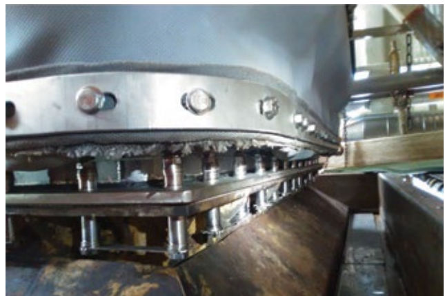
Siemens Energy. The company's life extension program for the LM2500 includes field repair solutions such as the flange upgrade shown here
