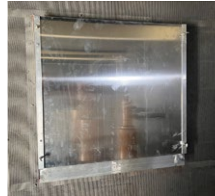
2. Open area to atmosphere is regulated by adjusting the position of the aluminum plate
