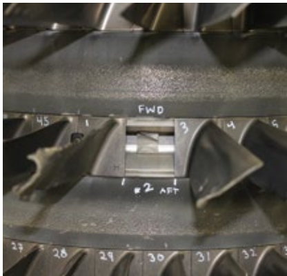
4. Edge-of-contact crack in the aft pressure face of Blade 2 in the fourth stage of the HP compressor was the root cause of this 2017 failure. The airfoil liberated while the dovetail remained in the spool. Coating was missing at the origination point of the crack with coating depletion leading to increased stress. The OEM said this was the industry's first reported failure of a dual-intensity peened blade (introduced in 2014 and installed that December)
