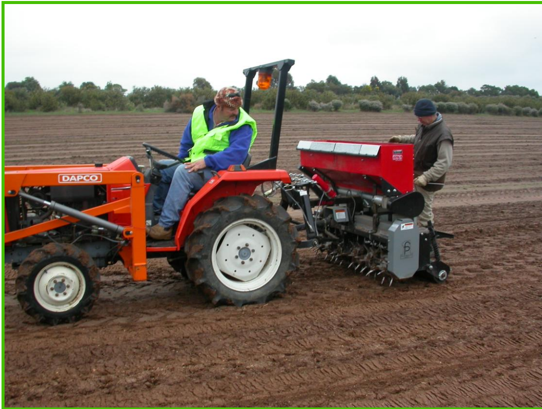
Figure 3: The modified turf seeder which allows the sowing of multiple species in one pass in action at the GGRP Chatsworth site (Glenelg-Hopkins CMA region).
