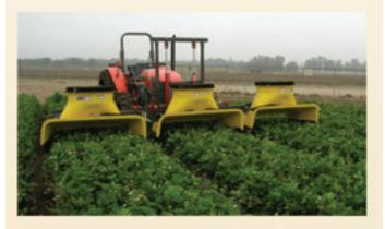
The fans raise and lower hydraulically as well as fold up for transporting. Hydraulic power comes from a PTO mounted pump with a self-contained hydraulic reservoir. PTO HP requirement is approximately 60 HP. We fabricate 3 and 4 row configuration from 48' to 68" beds.
