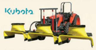
Designed to be LIGHT yet POWERFUL, the C&N Bug Vac is hydraulically powered with fans the develop 4700 feet per minute suction over the row. This sends all jumping and flying insects into the deflectors like bugs on a windshield.
