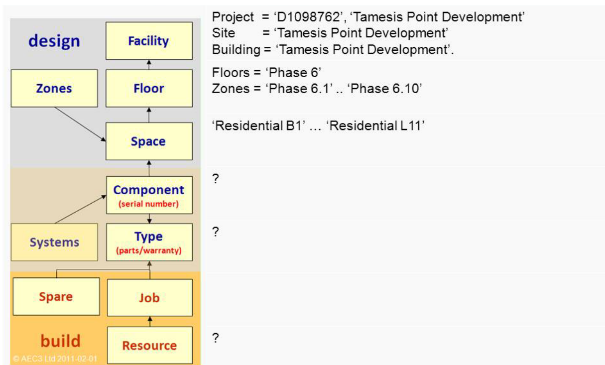
Mapping the overall structure of the master plan to COBie (AEC3). The land parcels such as 'residential b1' are documented as 'Spaces' and are then grouped to make up the main phase ('Floor') and subdivisions of the main phase ('Zones').
