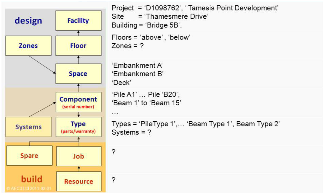
Mapping the overall structure of the Bridge to COBie (AEC3) Note that the physical 'Components' can be assigned to work areas ('Spaces') such as Embankment A.
