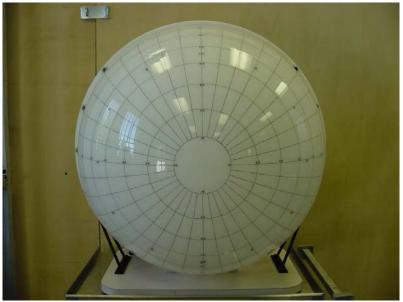
Figure 3. Graduated spherical shell or hemisphere
