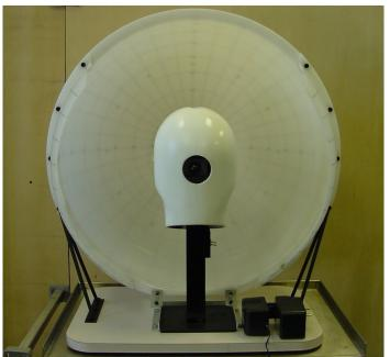
Figure 1. Stoll apertometer test fixture
