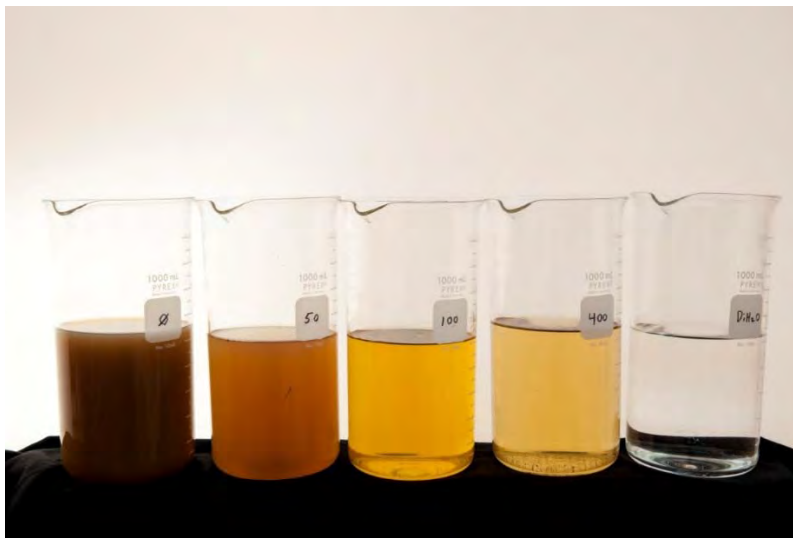
Figure 1. Effect of PAM at various rates (0, 50, 100, 400 g/m 3 on turbidity of soil leachate. Potting soil contained 15 percent sand and 85% organic products. Image here are of leachate collected after third irrigation. Deionized water on the far right for comparison.
