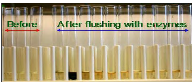
Figure 2. After a pulse of pure PG+EGase, the 20 nm gold particles pass through. The gold can be seen immediately after adding both enzymes, although it concentrates in the second fraction collected after the addition.
