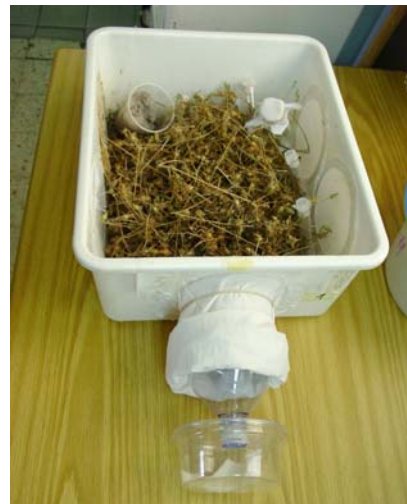
Figure 2. Opened horizontal cage, lid removed, used in capturing emerging insects.
