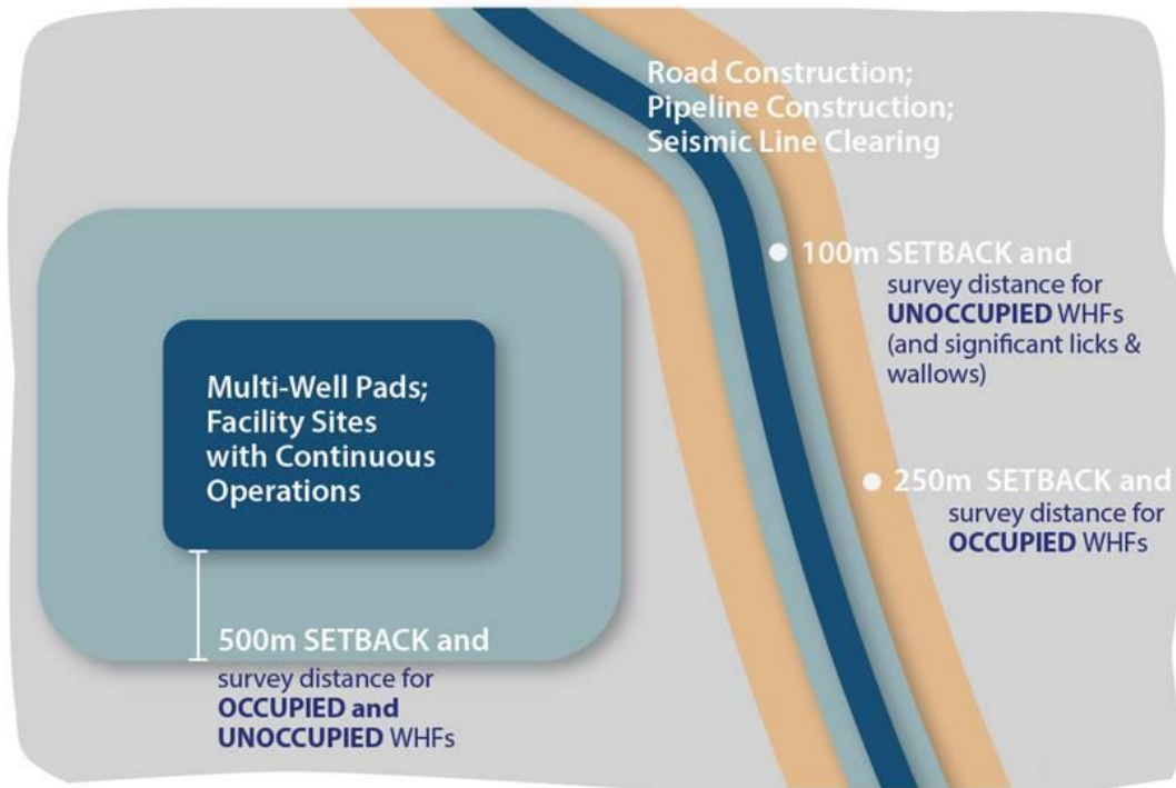
Figure 1.3: The application of setbacks and survey distances for oil and gas activities proposed within areas requiring WHF survey.
