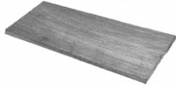
Figure 3a. Certi-Label western redcedar shakes. Used with permission from Cedar Shake & Shingle Bureau, New Roof Construction Manual .
