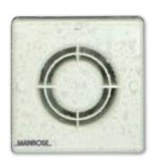
Suitable for mounting within the splash area of a shower or bath (where current regulations prevent the use of conventional fans), the 12 Volt fan is a standard model manufactured with a 12V - 50Hz shaded pole motor. The transformer and switching mechanism is mounted remotely either in the roof space or high on the ceiling next to the pullcord switch.
