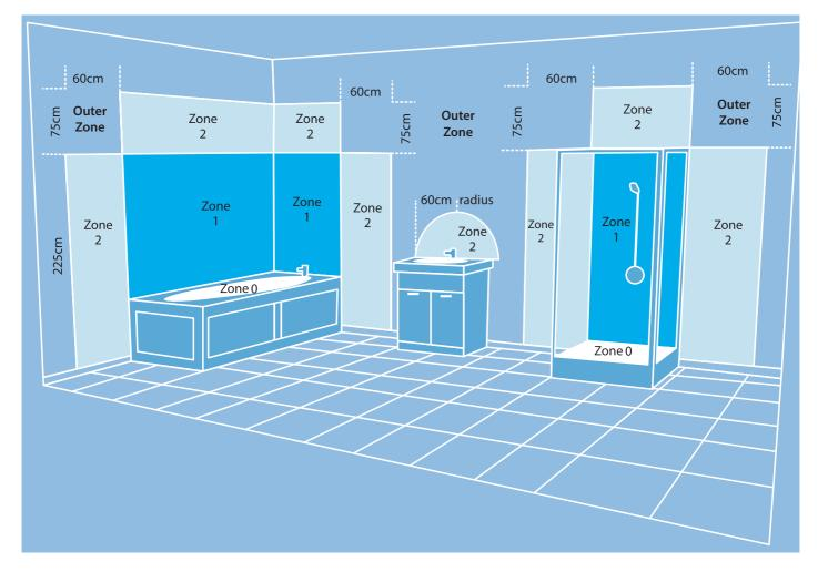
The following information is a guide to help you understand what fittings can be placed where in a bathroom. This is not an installation guide and reference should be made to the IEE Wiring Regulations 18th Edition (BS 7671:2018) or a qualified electrician.
