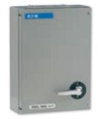
Exel 2 switch disconnectors and switch-disconnector fuses meet the constructional requirements for isolation of and are type tested to BS EN 60947-3. Switches are of the quick make and break type, suitable for use on AC or DC. Units have removable moving contact assemblies to facilitate wiring.
