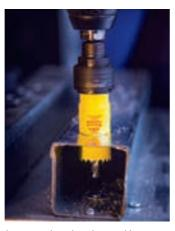
The Fast Cut saw combines a new tooth material, with enhanced heat and wear resistance, and a new tooth design, providing a smoother, faster cut on a wide range of materials, when compared against the previous Constant Pitch saw.
