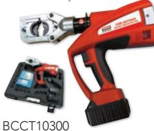
Battery operated crimp tool complete with hexagonal profile dies 10 - 300mm². Supplied with interchangeable cable cutting blades for copper and aluminium cable up to 40mm diameter (up to 70mm<sup>2</sup> 4 core PVC SWA/PVC Cable). Supplied with all dies, cutting blade, 2x li-ion 18V batteries and charger, carry case and strap.
