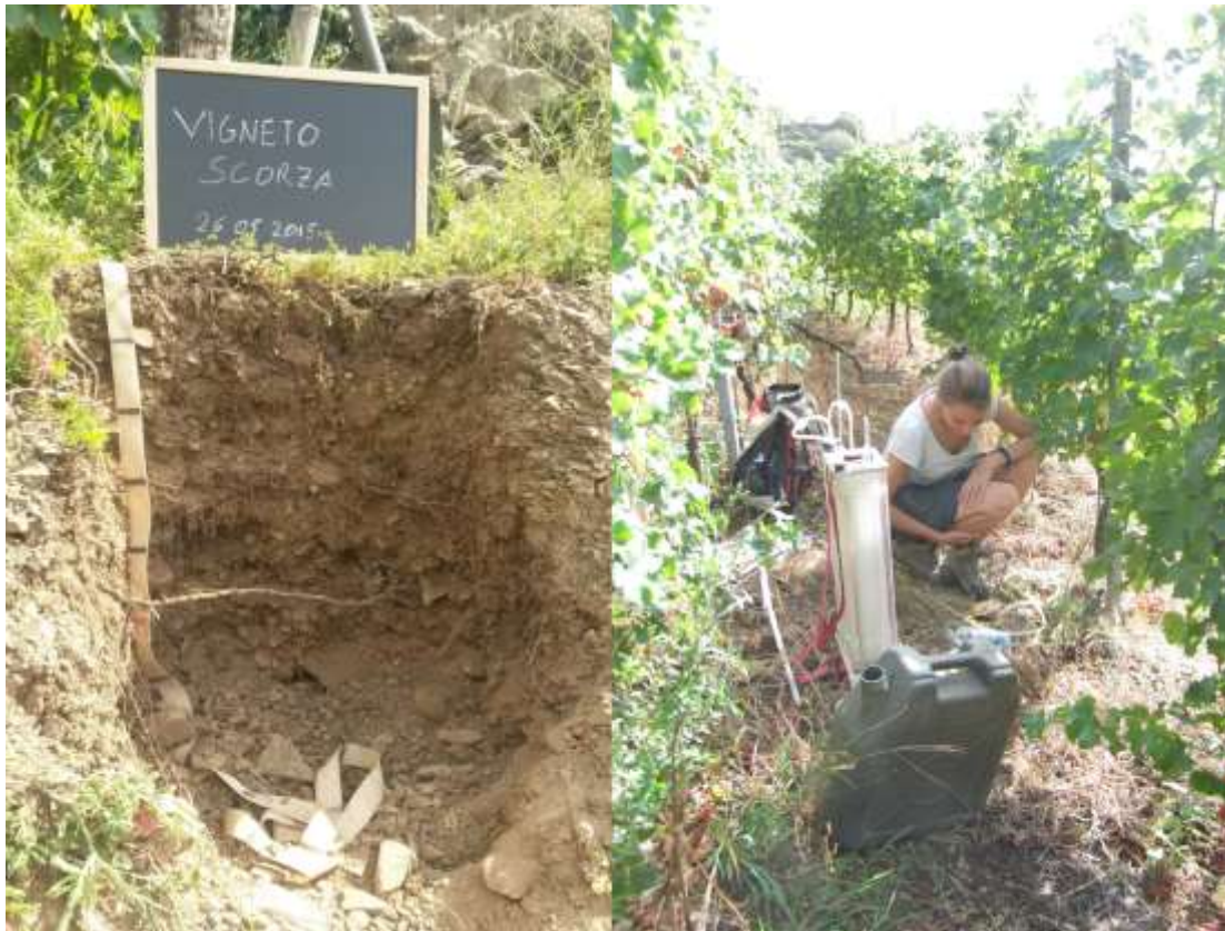
Figure 5: Example of a soil profile in a vineyard and measurement of soil hydraulic conductivity with an constant head permeameter (Amoozegar, 1989).
